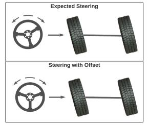
Figure 1.1: Illustration of a steering wheel offset in regard to the front axle of a vehicle. The top illustrates the relationship between steering angle and wheel position as expected. The bottom illustrates a steering offset. In this particular case of -15 degrees (to the left) for illustration purposes.
