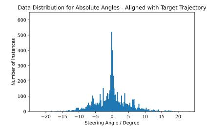
Figure 4.1: Histogram with bins of  $0.25^{\circ}$  width showing the distribution of data aligned with target trajectory. 6,055 Images - Mean:  $0.008^{\circ}$ - Standard Deviation:  $5.33^{\circ}$
