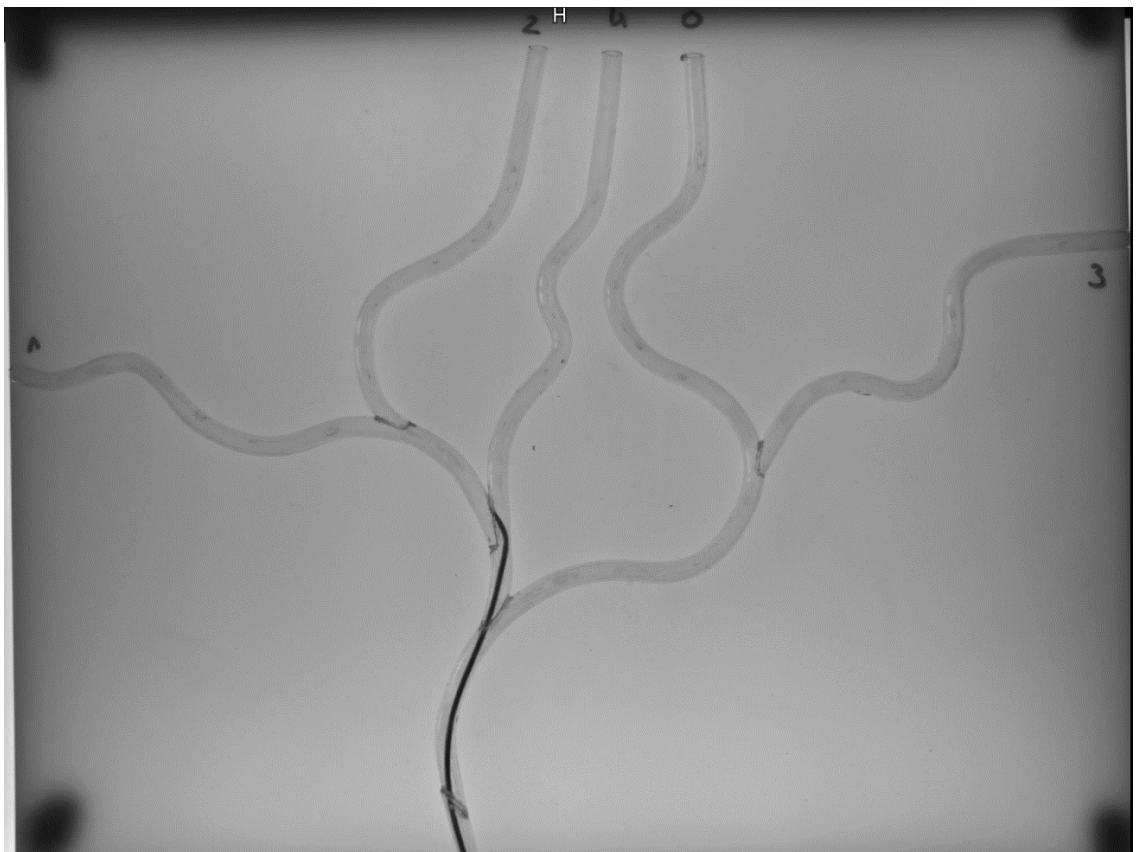
Figure 10: Camera recordings of a catheter moving inside an acrylic tubular structure. Used in this thesis for analysis of mechanical influences.
