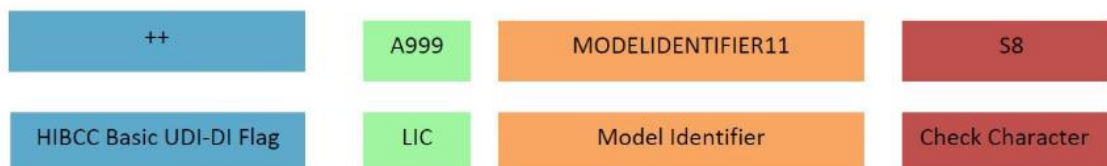
Fig. 10: Generating the Basic UDI-DI with HIBCC which is split into four parts [31]
