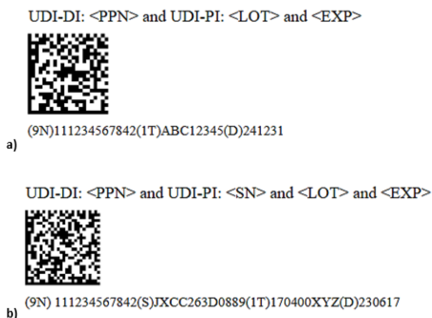
Fig. 5: Two Data Matrix codes with different UDI-PI information [25]
