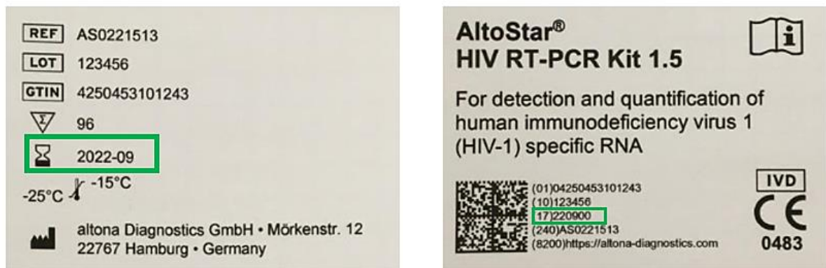
Fig. 21: On the left, the label "Symbole" where the date is only given with month and year. On the right, the date is displayed in the format YYMMDD in the UDI carrier. Two zeros are entered for the day, since no exact day is specified (Own development)
