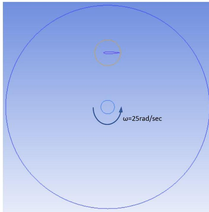
Figure 40 Angular Velocity of Rotating Domain containing Airfoil
