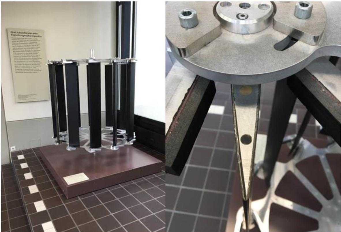
*Figure 6 Agile VAWT with Pitching Mechanism [3]*
