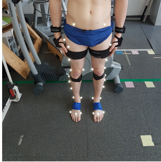
Figure 10: Subject with attached sensors and CAST marker set
