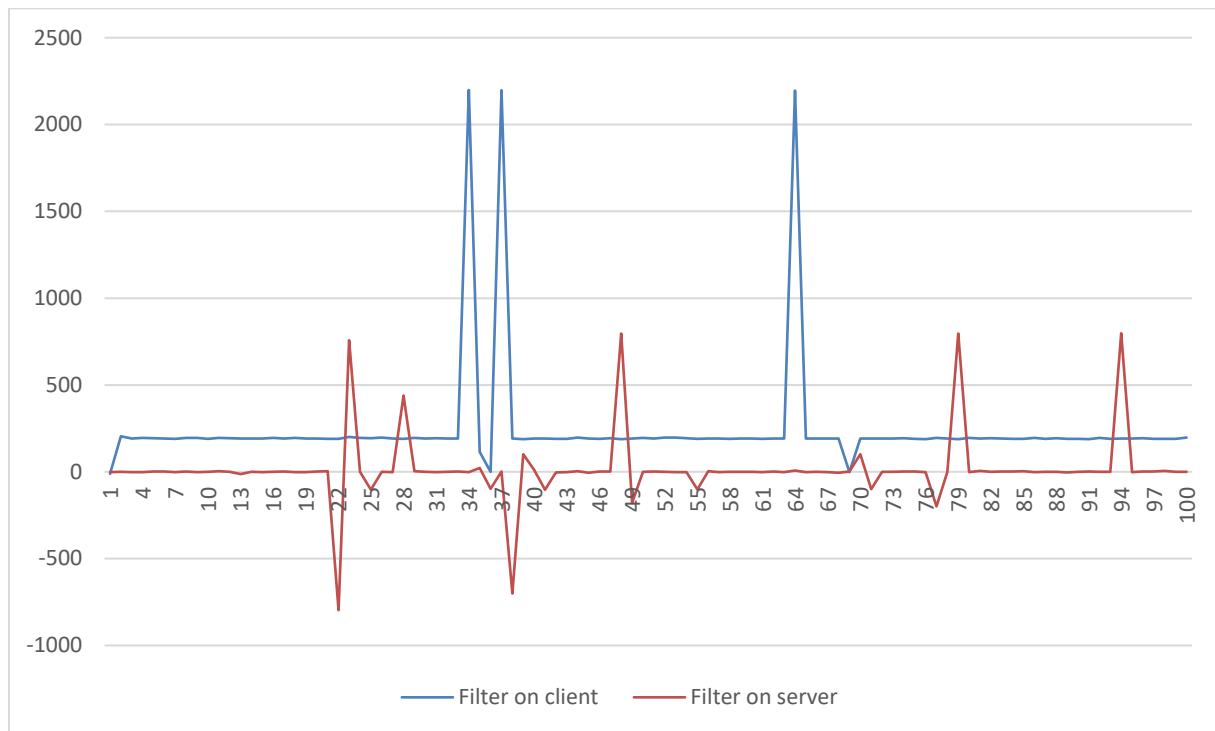
Figure 18 (One client and one server response time difference between caching enabled and disabled depending on the filter used on the client)
