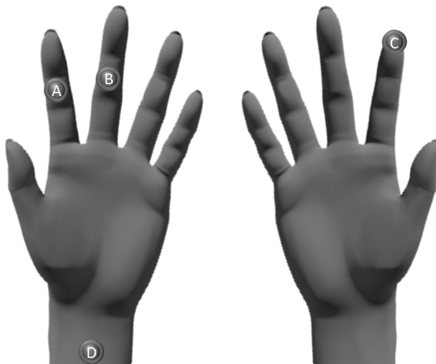
Figure 2.4: A: 1. EDA electrode, B: 2. EDA electrode, C: BVP sensor, D: 3-axis accelerometer
