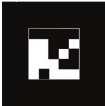
Figure 2.2: Example of a marker used in ARToolKit, a position calculation library [13]
