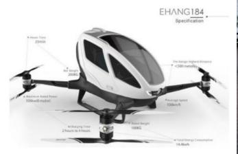
Ehang184 Carbon fibre monocoque 360kg 106kW
