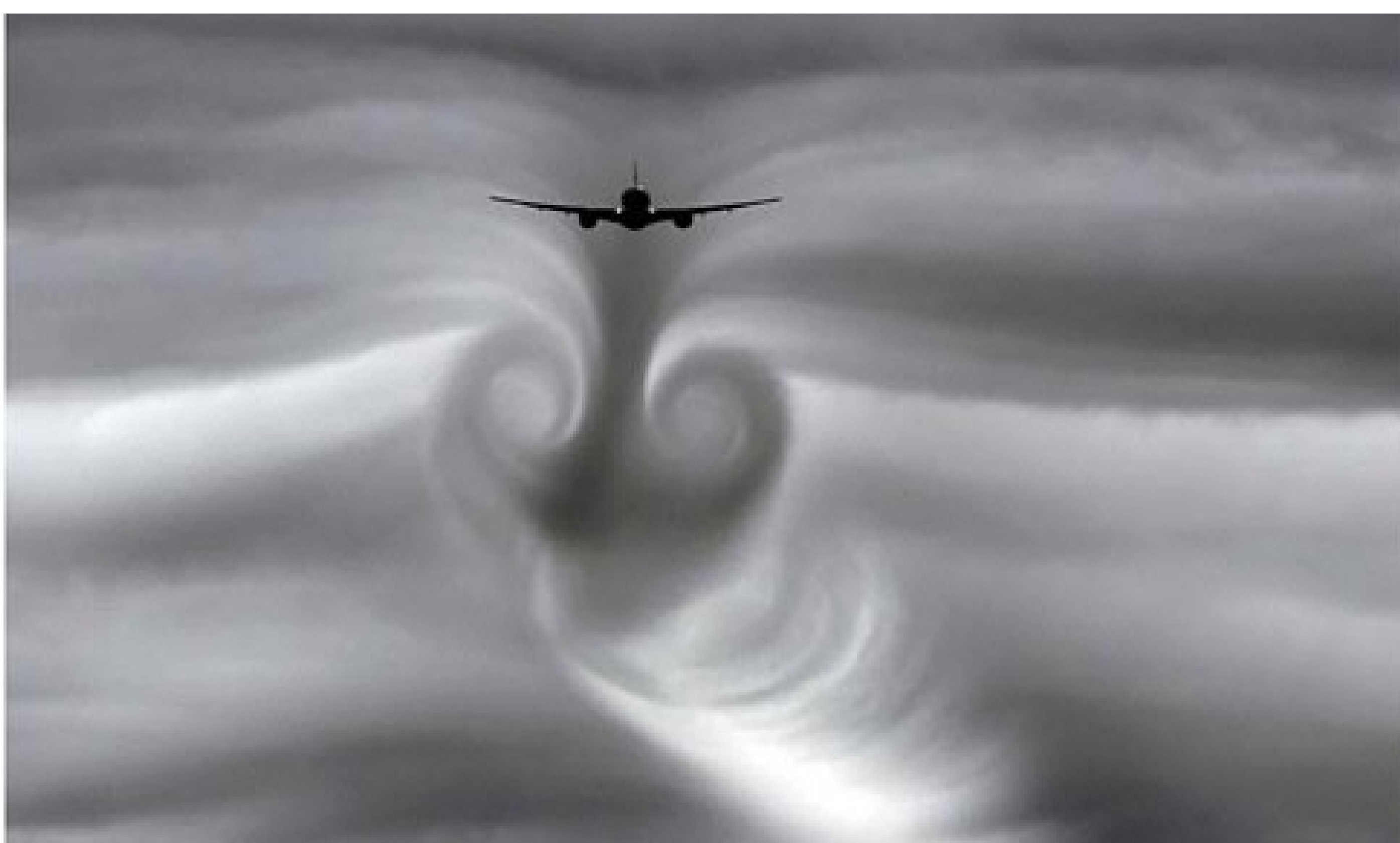
Figure 1: The vortex wake behind lifting wings descending through a thin cloud layer (Source: Airliners.net)
