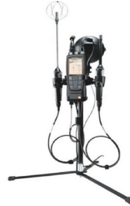
Testo-480 Device Mounted on Tripod for measurement
