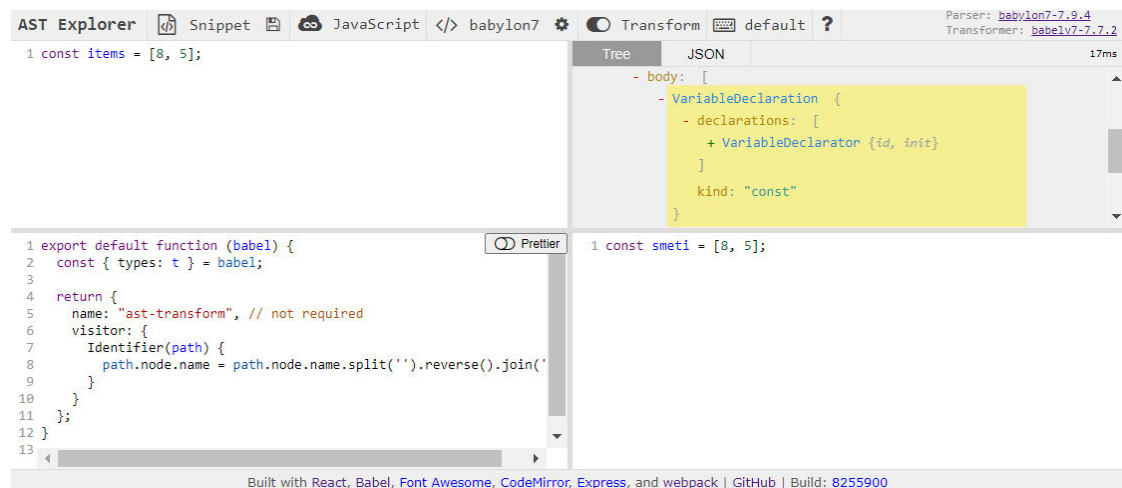
Figure 4.2: Screenshot of an abstract syntax tree transformation example taken from AST Explorer.
