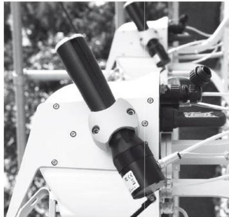
**PR1 SMART PYRANOMETER**
