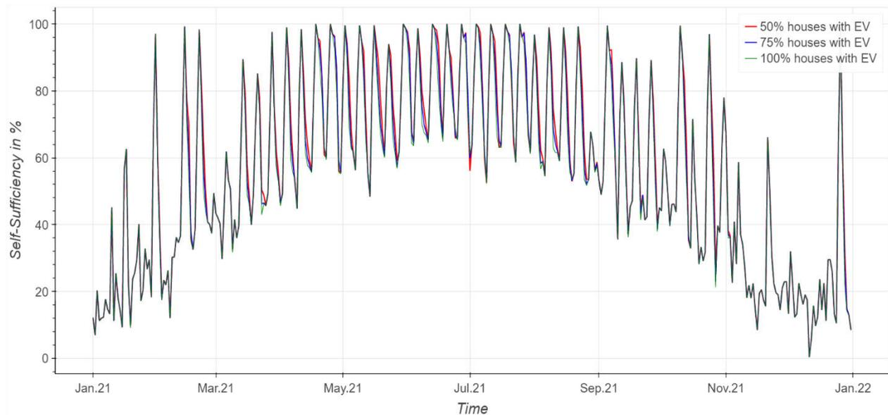
Figure 27 Self-sufficiency of PV system with EV as energy storage with different share of households owning EV
