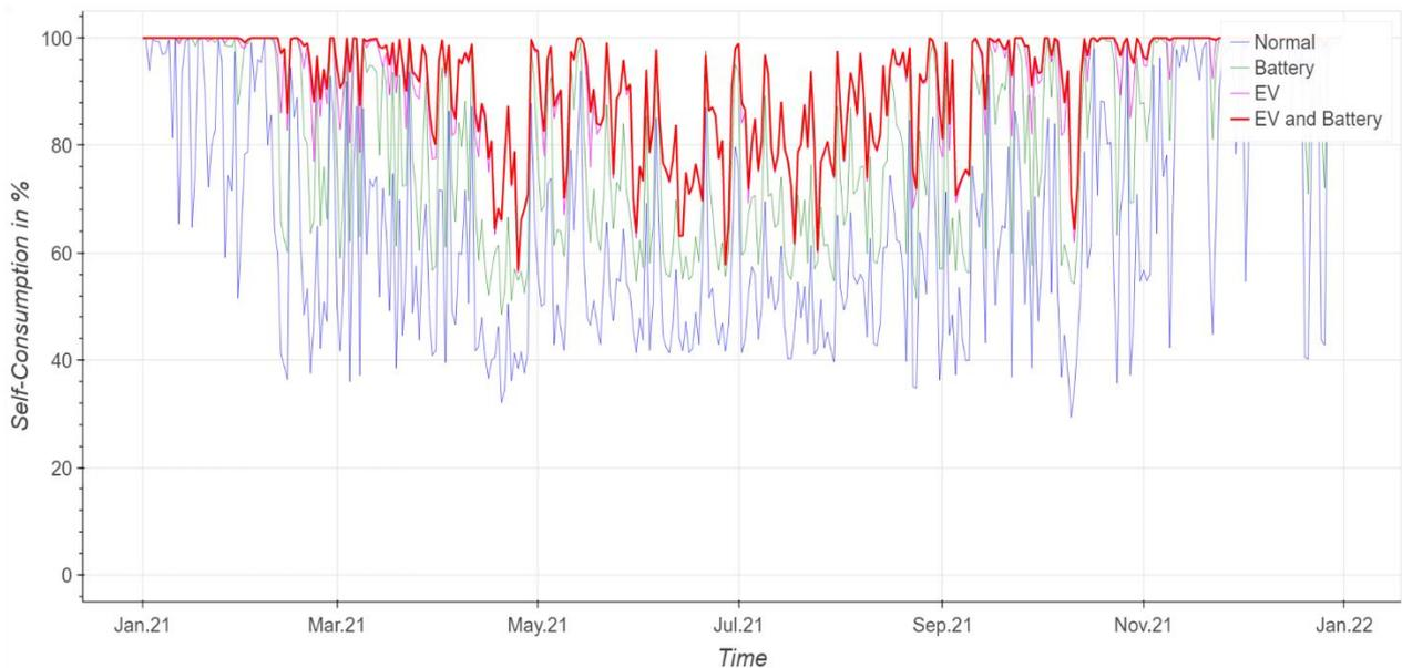
Figure 35 Self-consumption of residential PV systems in Hamburg with combination of EV and Battery as energy storage system
