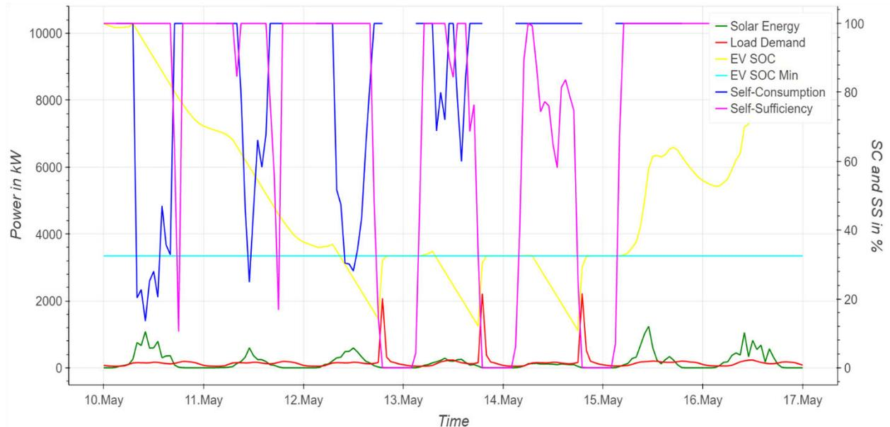
Figure 22 Analysis of SOC of the EV battery for validation of EV model
