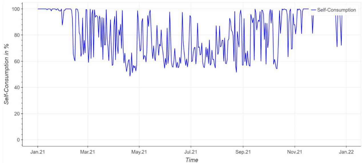
Figure 17 Daily average self-consumption of residential PV system with battery energy storage system
