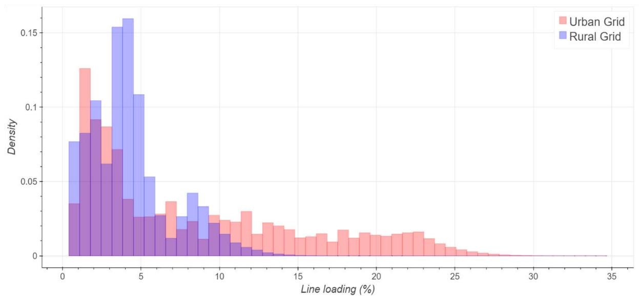
Figure 42 Comparison of line loading(%) distribution for urban(red) and rural(blue) grid considering EV and Bat model
