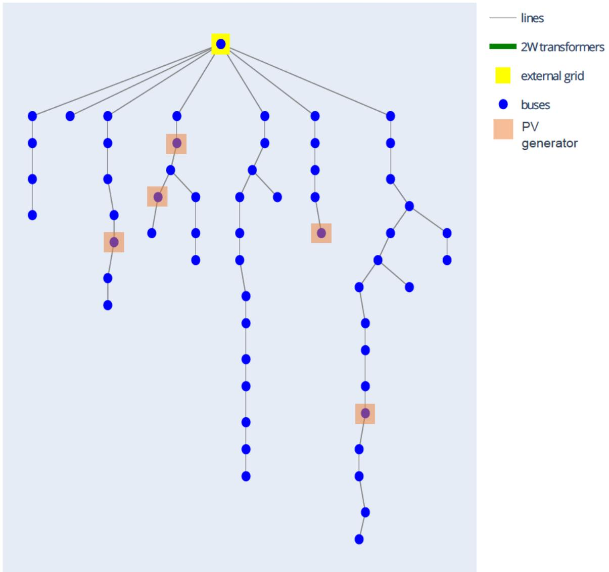
Figure 10 Grid structure of benchmark grid '1-LV-urban6--0-no\_sw\_test'
