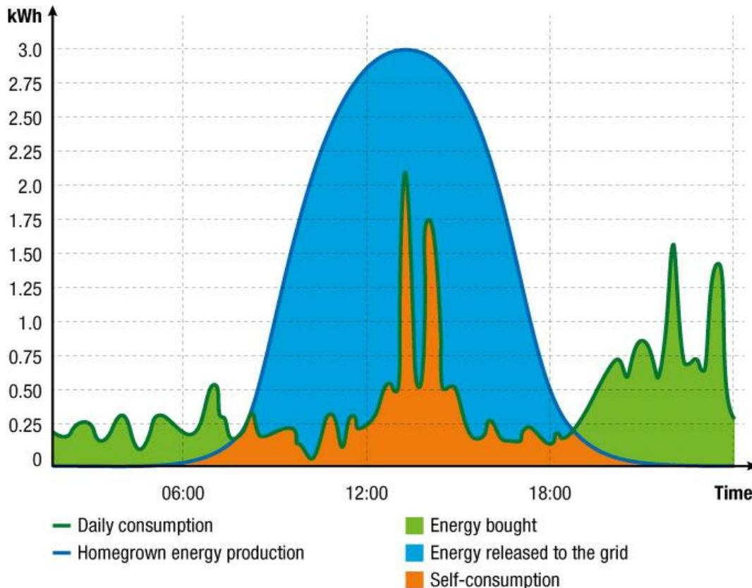
Figure 2 Schematic of self-consumption of PV system [79]
