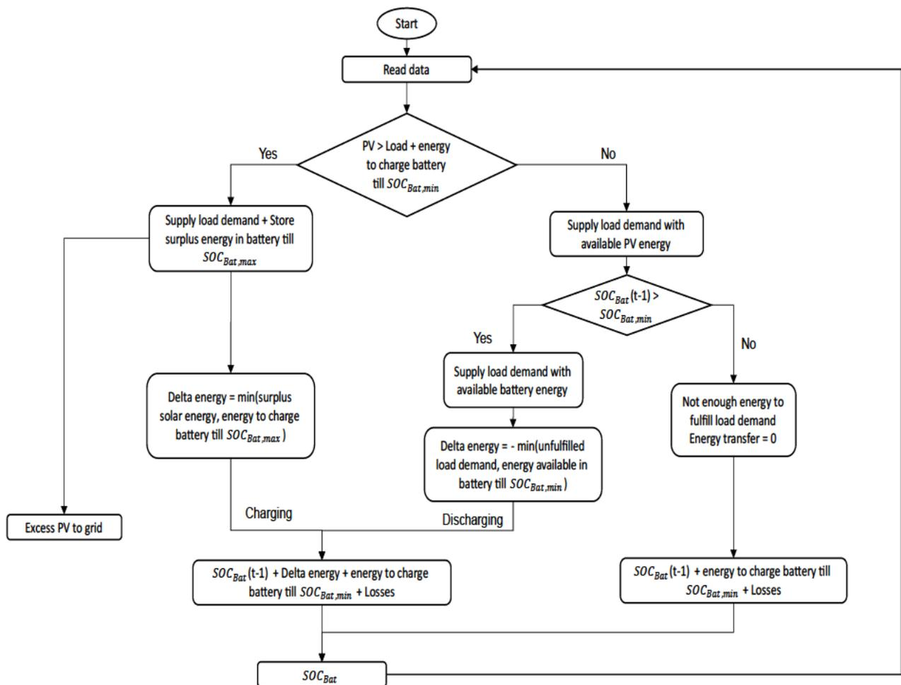
Figure 5 A flowchart of the battery energy storage system simulation
