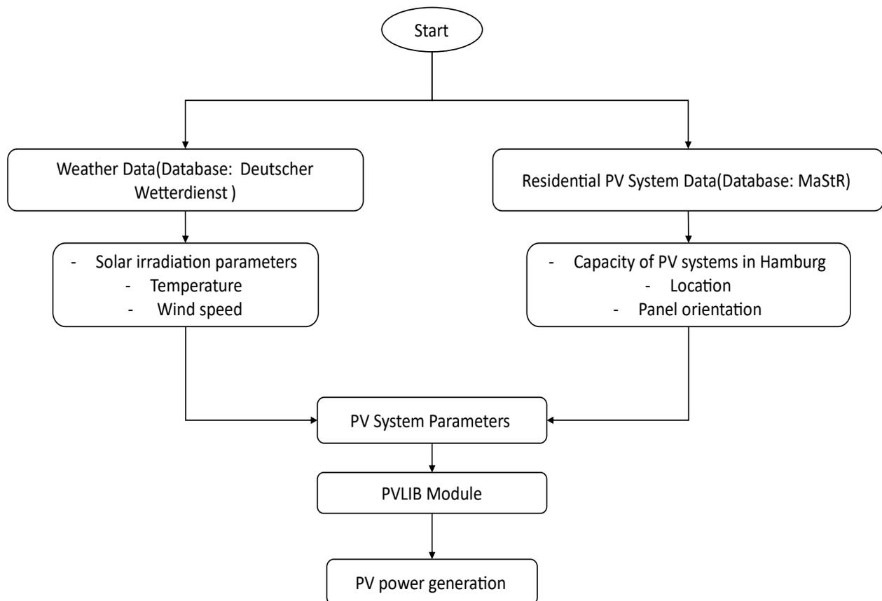
Figure 4 A flowchart of the PV power model
