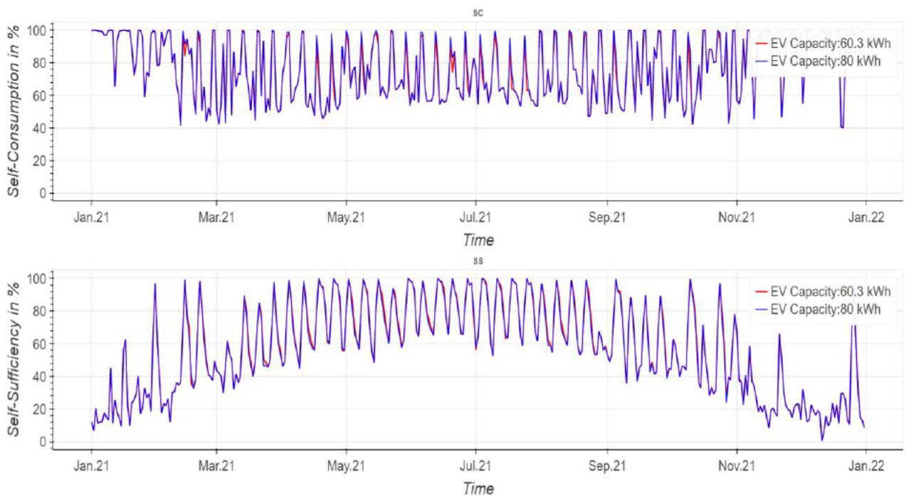
Figure 29 Daily average SC and SS of the system with two different average EV battery capacities with 50 % of household owning EVs
