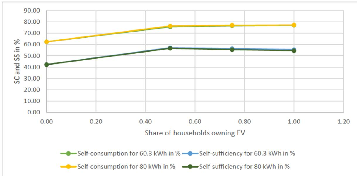
Figure 28 Analysis of SC and SS of the PV system with EV energy storage for different number of households owning EVs and different average EV battery capacity
