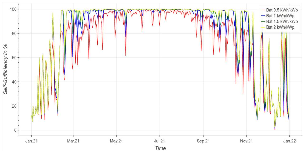
Figure 20 Comparison of daily average SS of residential PV system with different battery storage size
