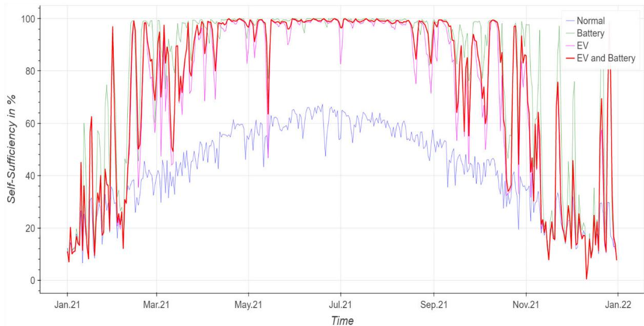
Figure 36 Self-sufficiency of residential PV systems in Hamburg with combination of EV and Battery as energy storage system
