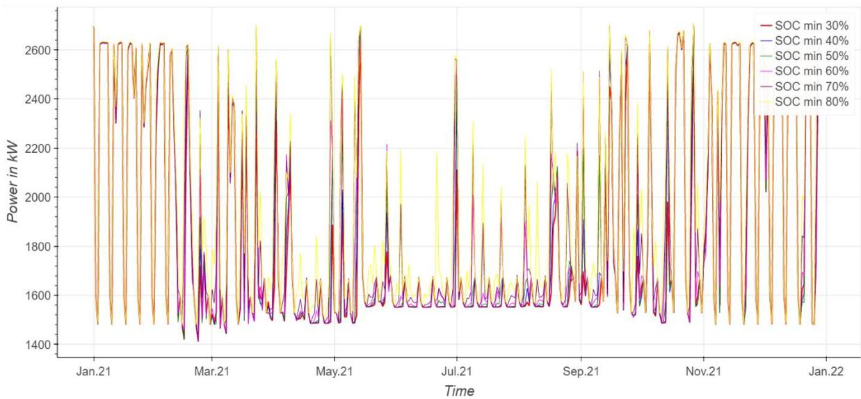
Figure 34 Load demand profile of the system with varying value of minimum SOC of EV
