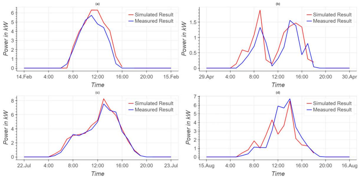
Figure 12 Solar energy generation profile of PV system in Energy Campus, Bergedorf (Red : Simulation output, Blue : Measured output) (a = 14<sup>th</sup> Feb, b = 29<sup>th</sup> Apr, c = 22<sup>nd</sup> July, d = 15<sup>th</sup> Aug)
