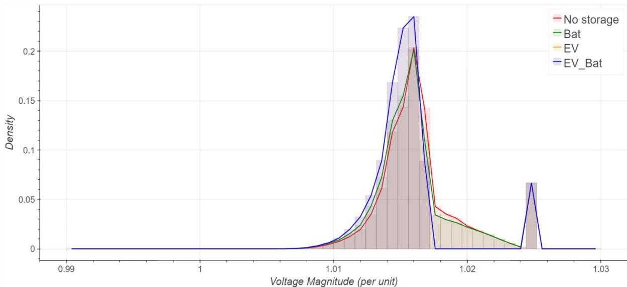
Figure 37 Voltage(per unit) distribution for all simulation models representing rural grid
