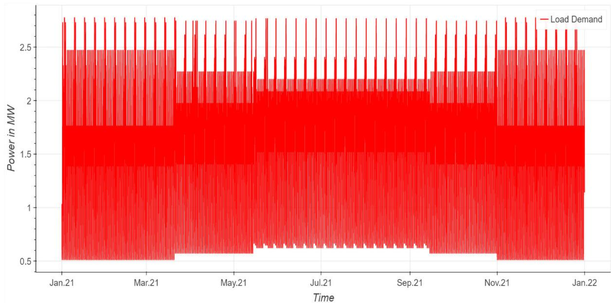
Figure 11 Load demand profile of households with PV system in Hamburg
