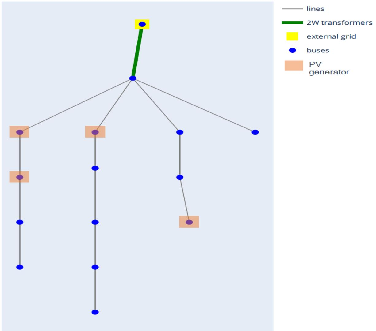
Figure 9 Grid structure of benchmark grid '1-LV-rural1--0-no\_sw\_test'
