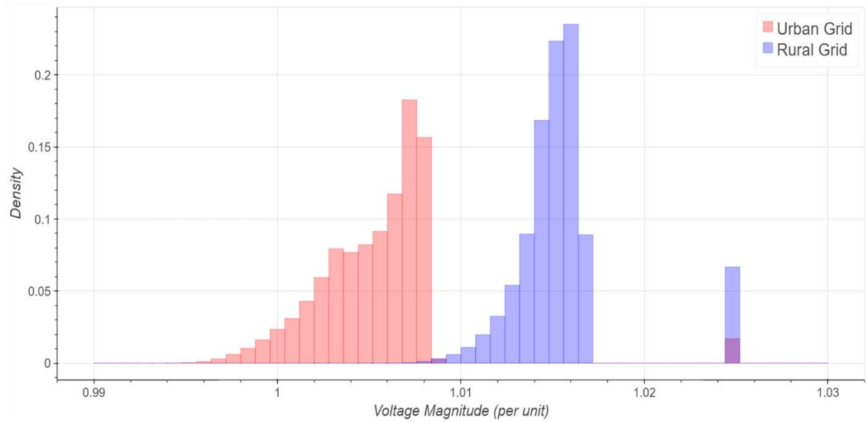
Figure 41 Comparison of voltage(per unit) distribution for urban(red) and rural(blue) grid considering EV and Bat model
