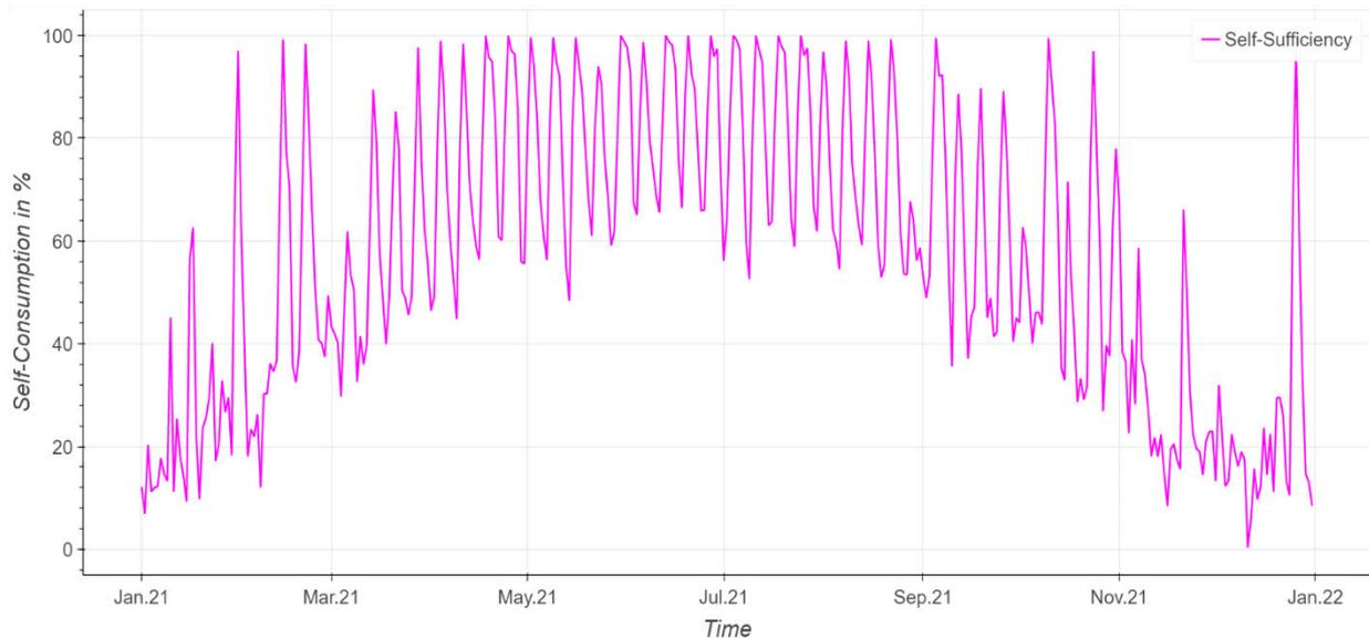
Figure 25 Daily average self-sufficiency of residential PV system with EV as energy storage system
