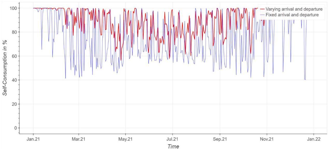
Figure 31 Self-consumption profile of the PV system using EV with varying departure and arrival behaviour
