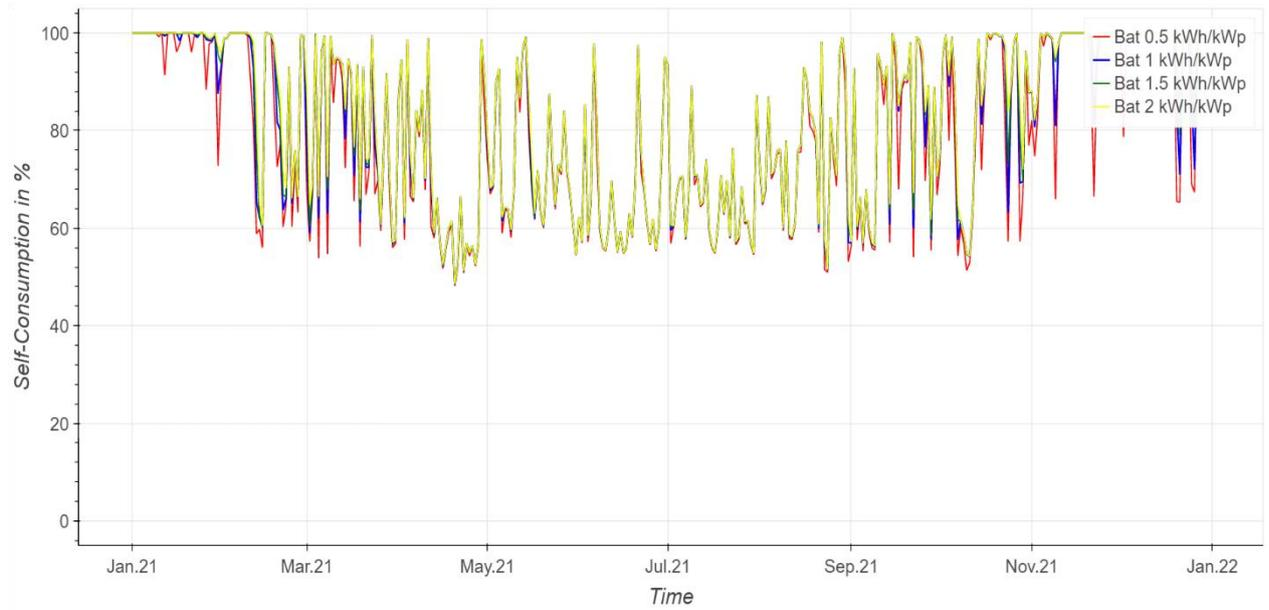
Figure 19 Comparison of daily average SC of residential PV system with different battery storage size
