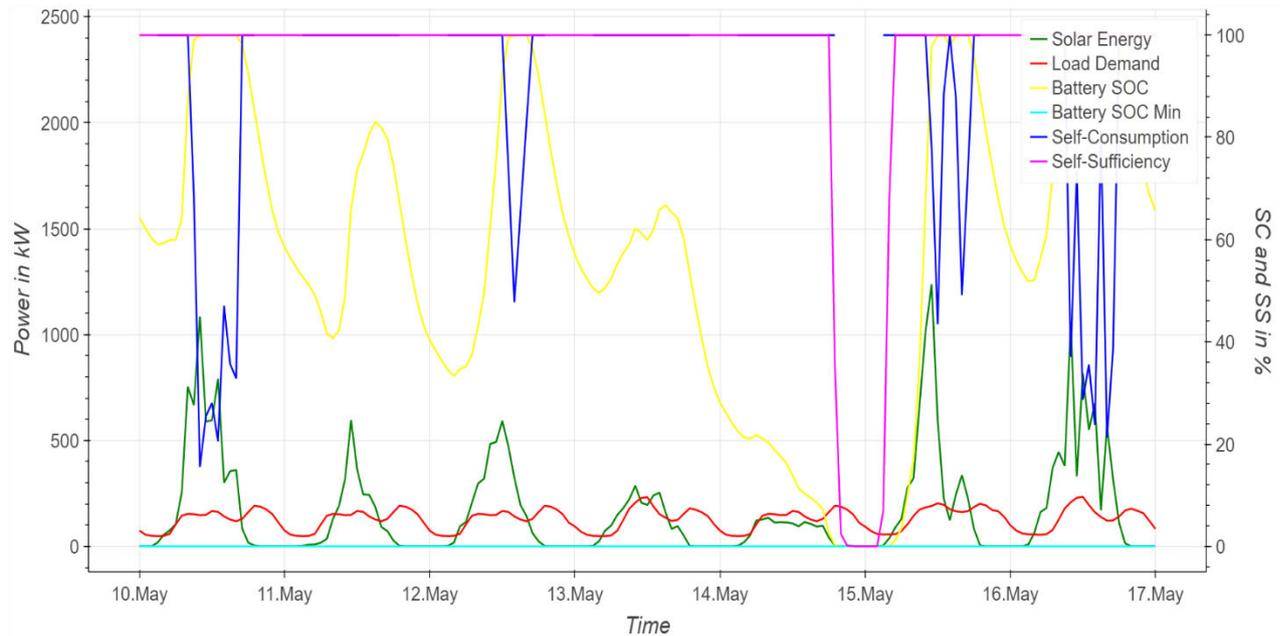
Figure 16 Analysis of SOC of the battery for validation of battery model
