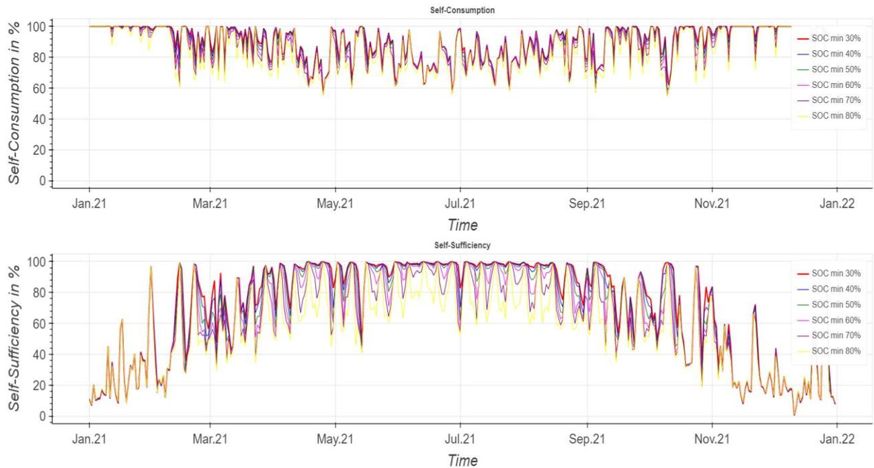
Figure 33 Daily average SC and SS of the system with varying value of minimum SOC of EV
