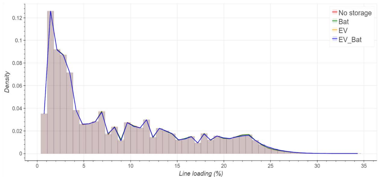
Figure 40 Line loading(%) distribution for all simulation models representing urban grid
