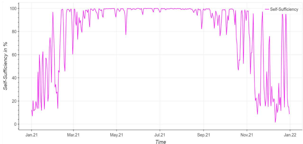
Figure 18 Daily average self-sufficiency of residential PV system with battery energy storage system
