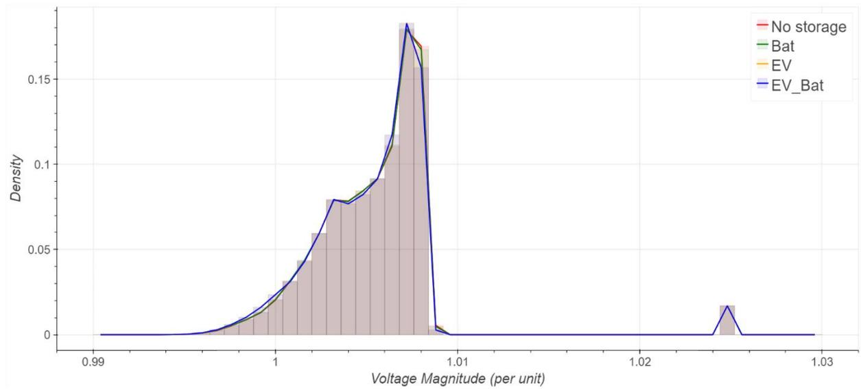
Figure 39 Voltage(per unit) distribution for all simulation models representing urban grid
