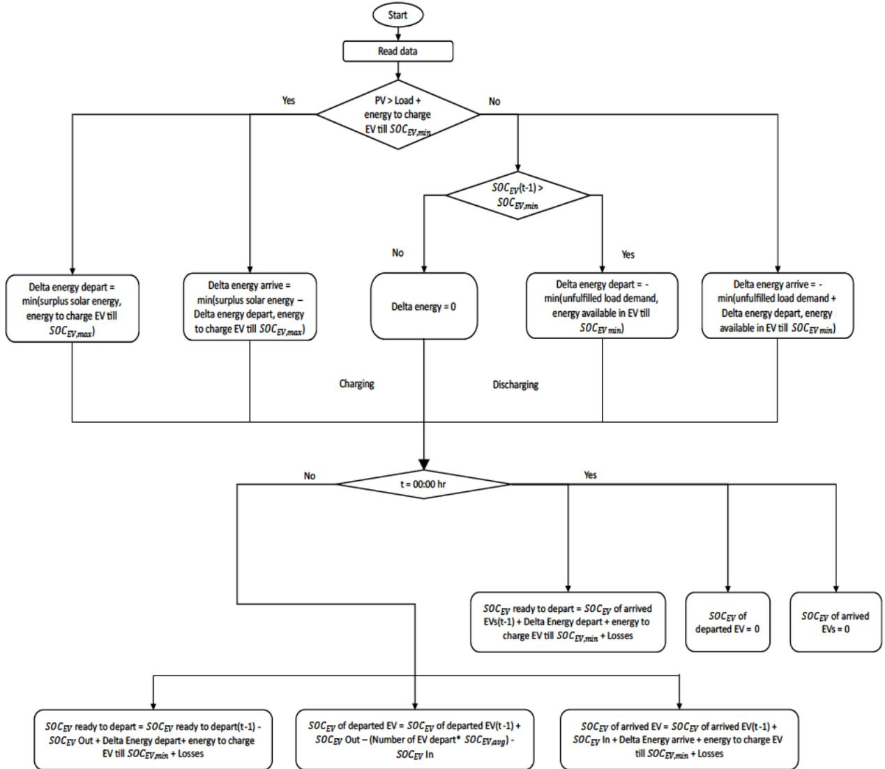
Figure 8 A flowchart of EV energy storage simulation model with arrival and departure time of EVs
