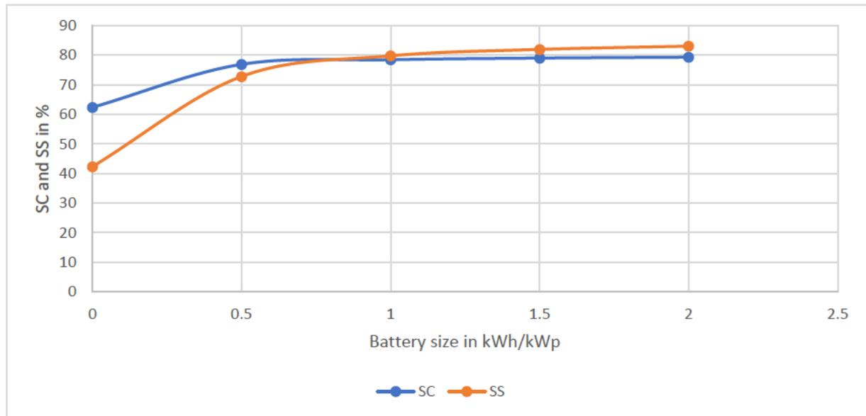
Figure 21 Analysis of degree of SC and SS for varying size of battery capacity per kWp
