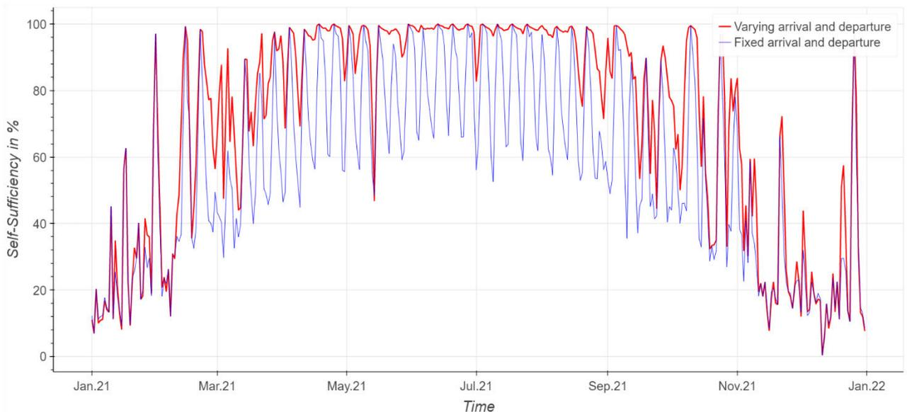
Figure 32 Self-sufficiency profile of the PV system using EV with varying departure and arrival behaviour
