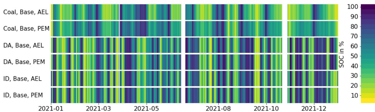
Figure 7.13: Optimized dispatch of the St represented by the St_SOC variable in the year 2021 for the three energy-markets and both El technologies.
