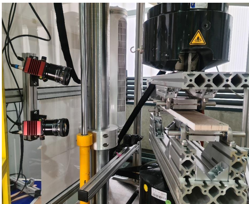
Figure 41: four-point bending test setup with installed DIC system
