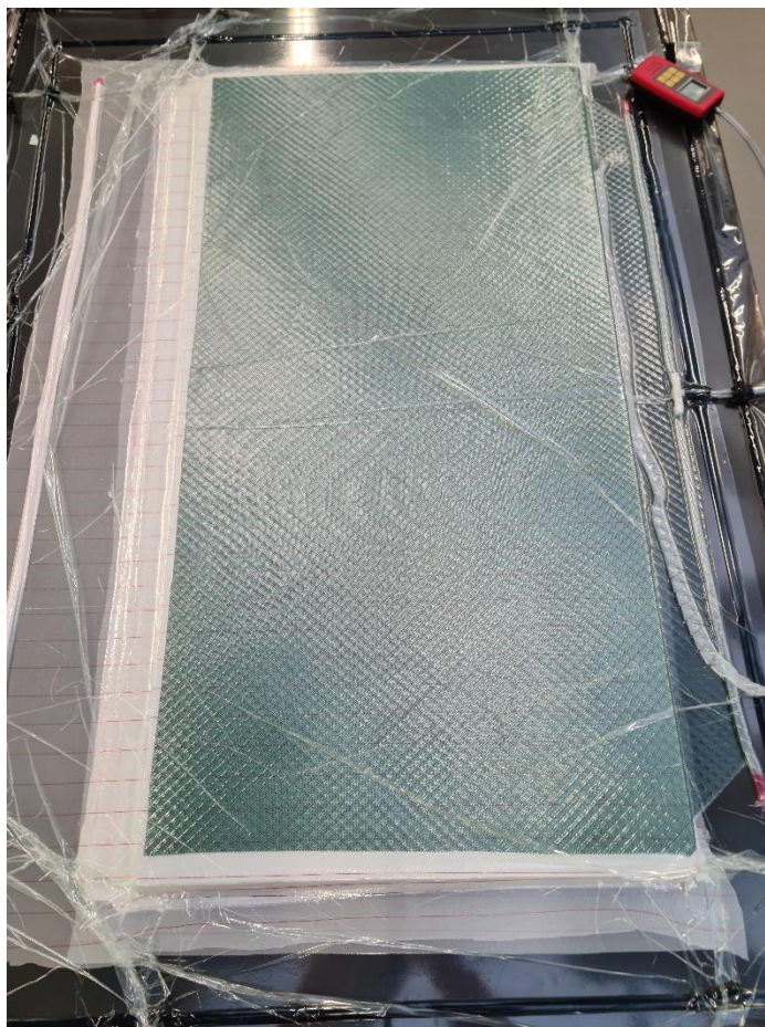
Figure 40: VARTM panel manufacturing with two vacuum bags
