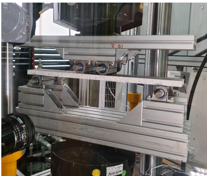
Figure 37: four-point bending test rig according to ASTM C393
