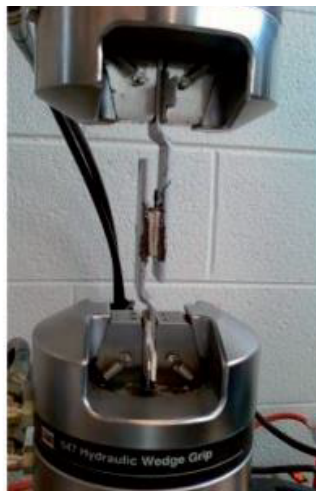
Figure 10: lap shear test setup Newaz et al. [23, p. 212]
