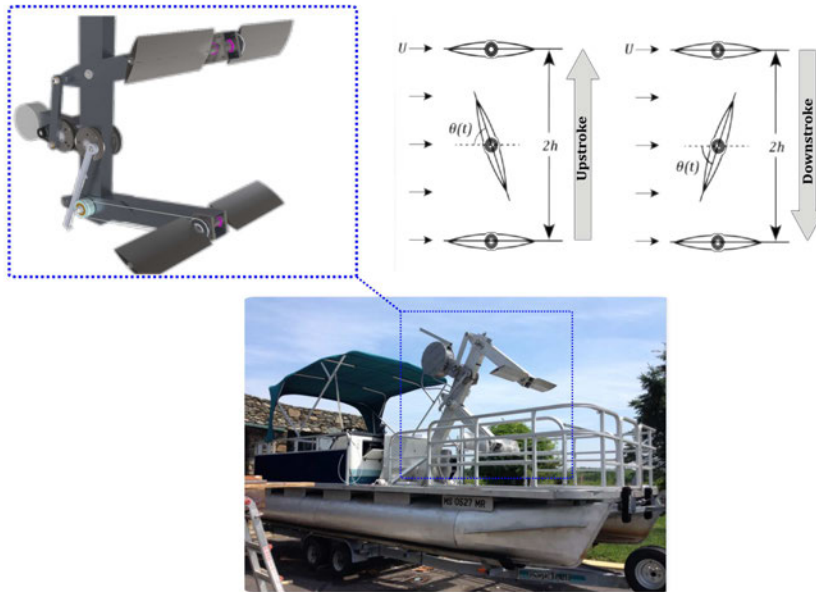
Figure 1.1: Energy harvesting oscillating hydrofoil system [6]. (Top-left) the CAD-model. (Top-right) the motion mechanism. (Bottom) the real design mounted on top of a pontoon boat for transit reasons.
