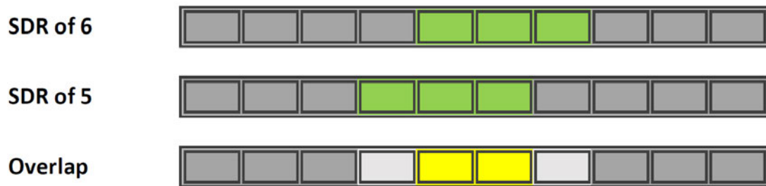
Figure 2.3: Encoding of scalar values into a 10 bit long SDR with a number of 3 active bits and a resolution of 1. Deliberately overlapping nearby values creates a meaning of similarity.
