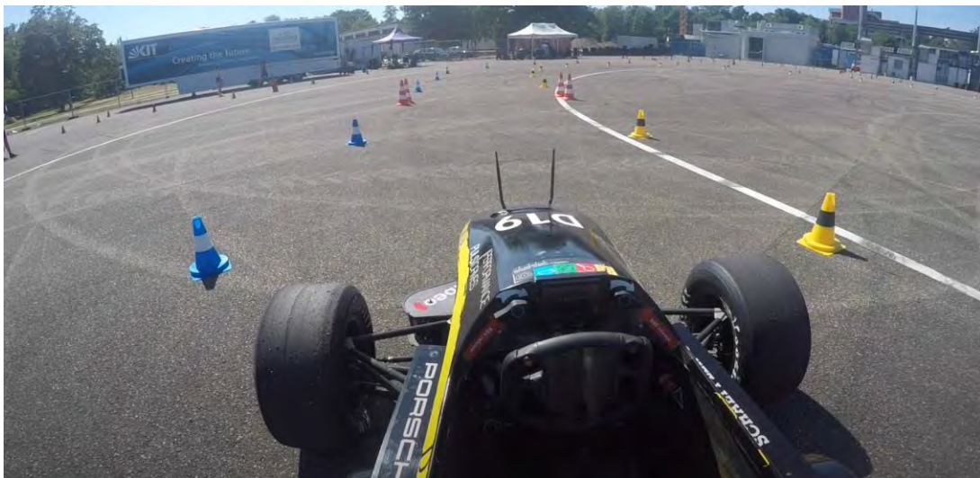
Figure 23: The image shows the driverless vehicle from KA-Racing during testing on an Autocross/Trackdrive racetrack [42]
