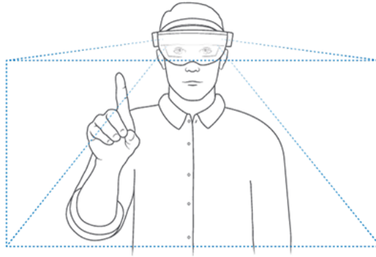
Figure 10. The gesture frame in which the HoloLens recognizes the hand is shown. [51]
