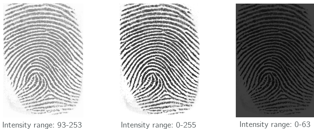
Figure 8.11: INV9 - Examples of gray-scale normalization to a desired range, fingerprint images are based on [Mai+02a, DB2]
