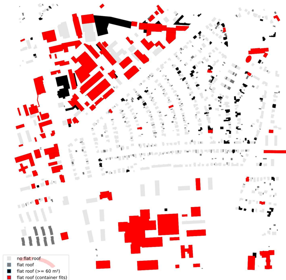
Figure 9: An exemplary tile with filtered buildings according to a flat roof structure that fits one DAC plant container module. The light grey forms are buildings with another roof structure. The forms in the darker grey color are flat roofs with a size smaller than 60 m 2 . Black-colored buildings are equal to or larger than 60 m 2 , however, they do not fit a polygon of the dimension of a common container. Red-colored buildings fit the necessary dimensions. (Trosdorff, 2023)
