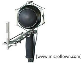
**Figure 3-5: Microflown devices for the in situ measurement of absorption coefficients**
