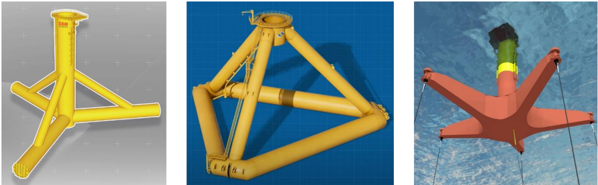
Figure 17: TLP concepts (from left to right): Float4Wind from SBM, PelaFlex from Marine Power Systems, Pelastar from Glosten [62], [63], [64]
