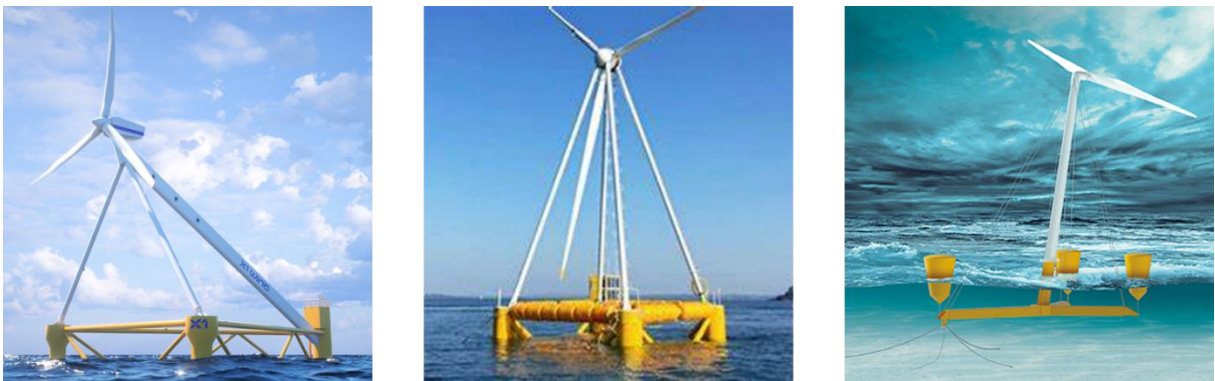
Figure 19: Self-aligning concepts (from left to right): X1 Wind from X1 Wind, Eolink from Eolink, Nezy from Aerodyn [70], [68], , [69]
