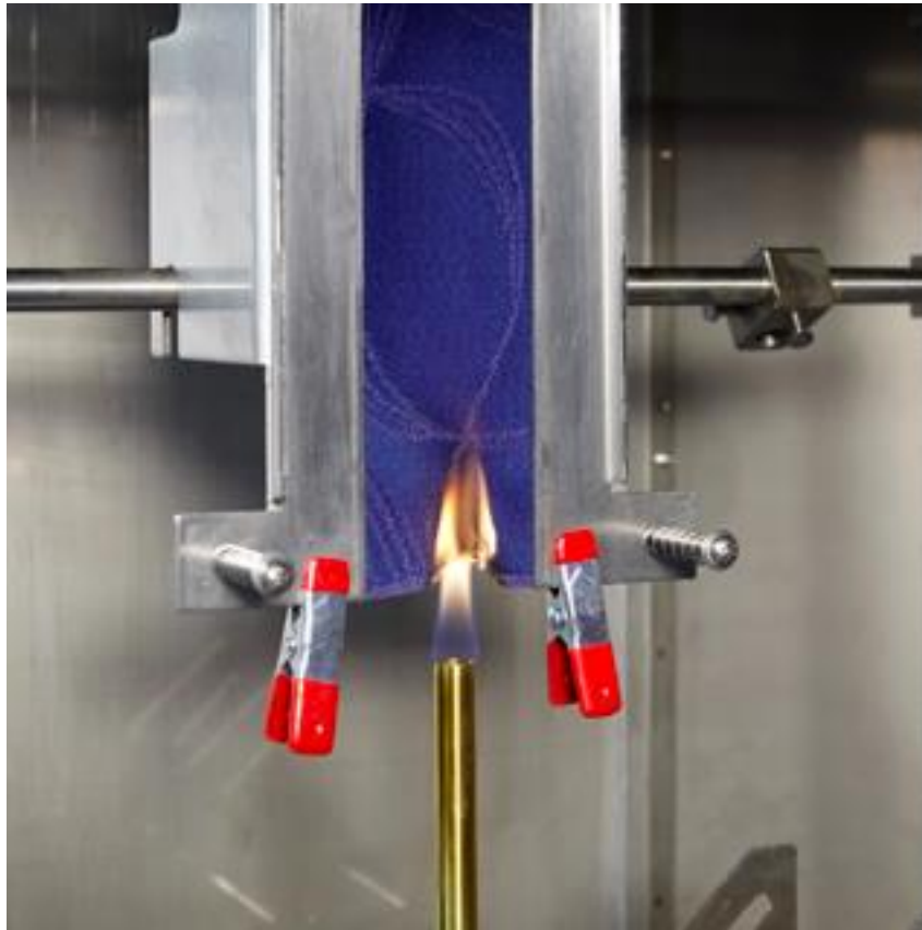
Figure 5-2: Vertical Bunsen Burner Test for 60/12 seconds, (AeroBlaze 2022)
