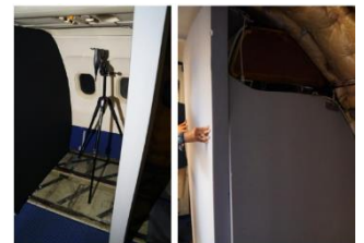
Figure 6 : Sound pressure measurement in Bear cave on panel without carpet.
