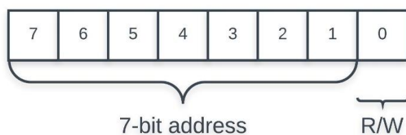
Figure 5: 7-bit slave address plus read/write bit
