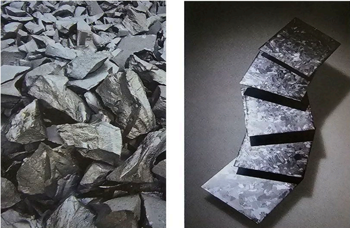
Abbildung 2-7 - Links: Polykristallines Rohsilizium. Rechts: Polykristallines Siliziumwafer. [Qua10]
