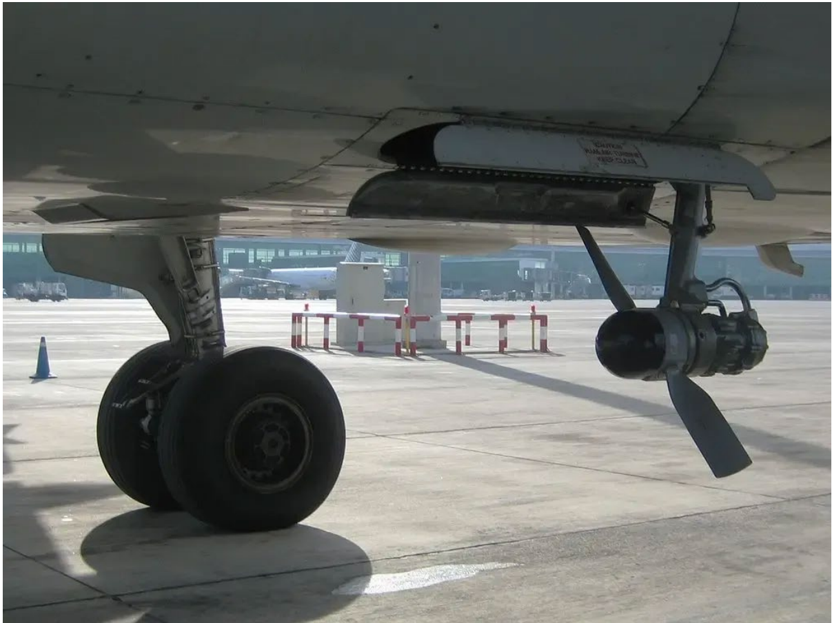
Abbildung 2-17 - Ram Air Turbine von Airbus A320 [Amr21]
