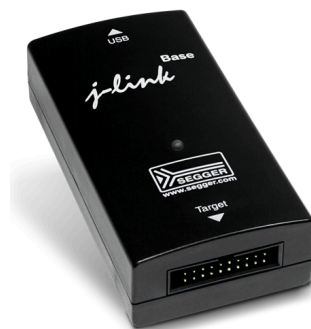
Figure 5.10: SEGGER J-Link Debugger from [15]
