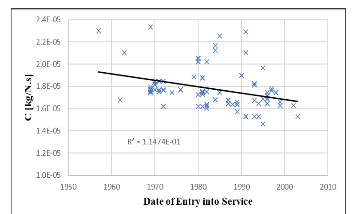
Figure 3: Future trends: SFC improvements with BPR are less pronounced with high BPR. Yes, SFC has been reduced over the decades (by 0.33% p.a.), but this trend is not that clear for all engines.
