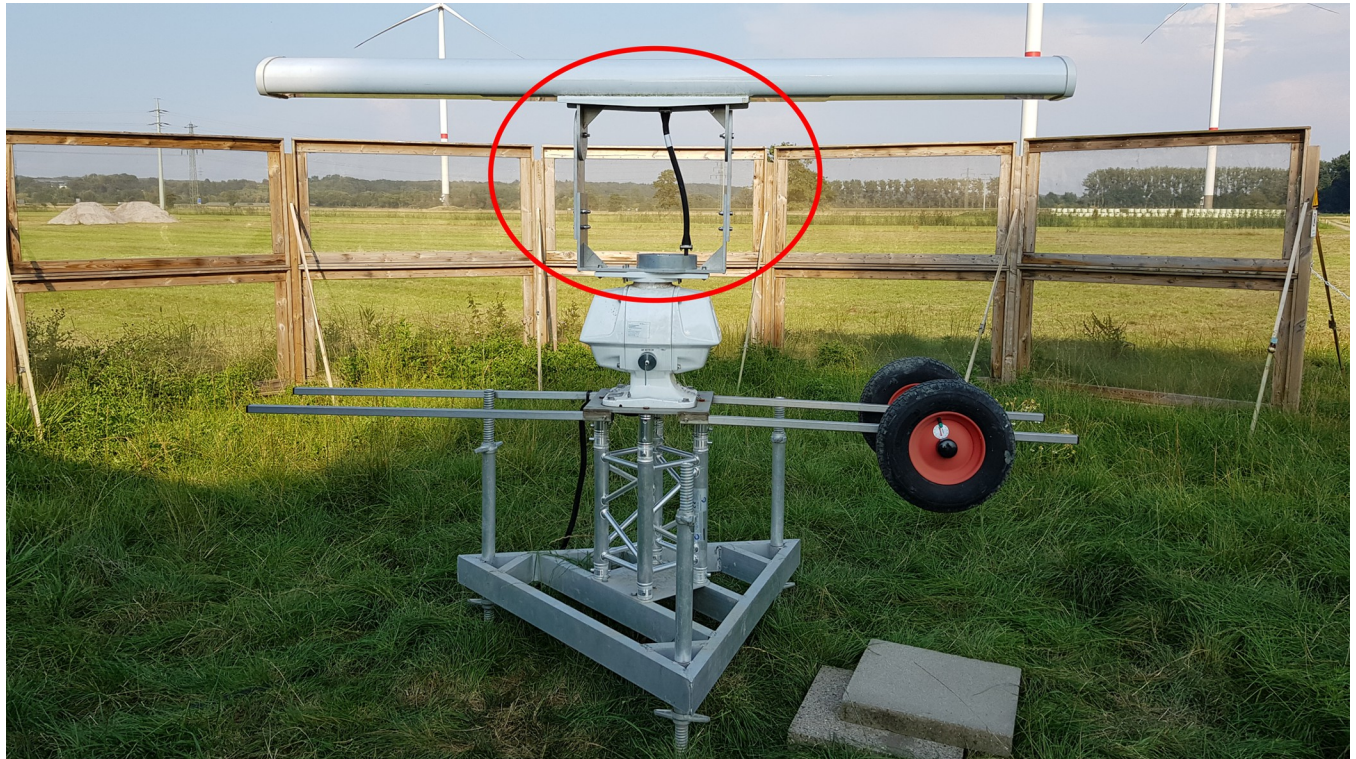
Fig 1. Modified FURUNO FAR 2117 marine radar setup used in this study. The red oval indicates the modified part of the radar—the waveguide in between aluminum panels for a custom adjustable vertical angle of the antenna. The clutter shielding fence is visible behind the radar, with three towers of the wind turbines in the background.
