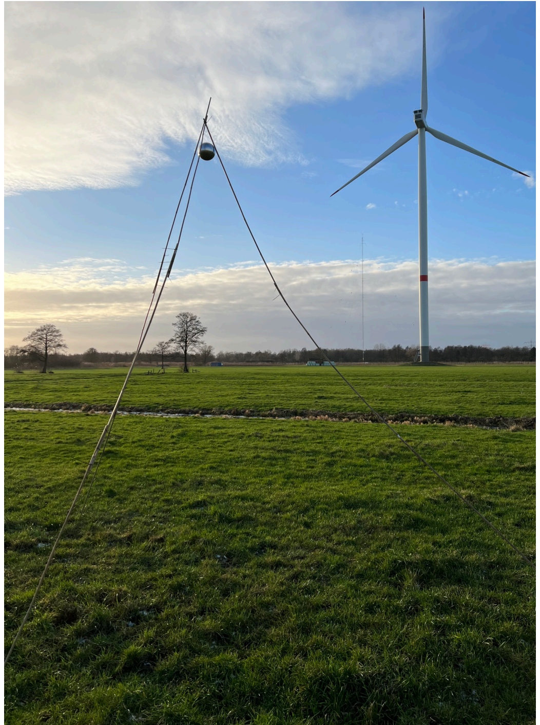
Fig 4. Field measurements of intensity levels of metal spheres with known RCS. Tripod, made from thin, dry bamboo rods, holding a polished hollow aluminum sphere of 150 mm diameter.
