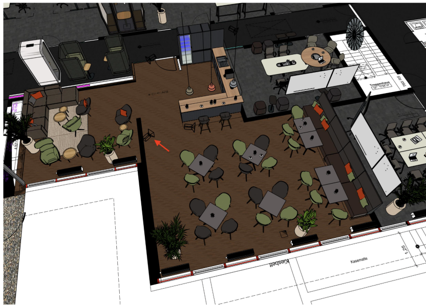
Figure 2.1: Design of the Work Café environment with the arrow indicating the position of the Kinect v2 camera
