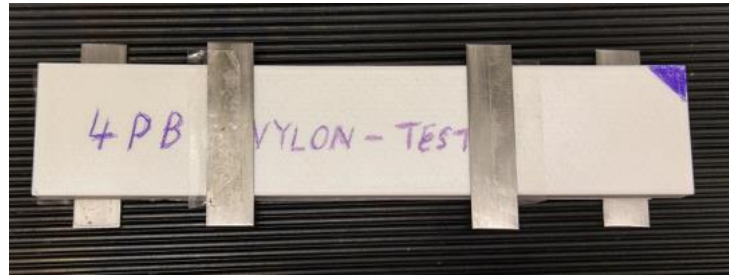
Figure 7-5: Metal sheets attached on the specimen
