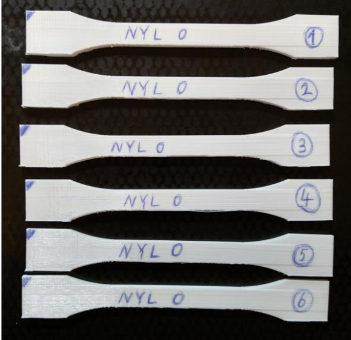
Figure E - 1: Printed "0°" nylon specimens
