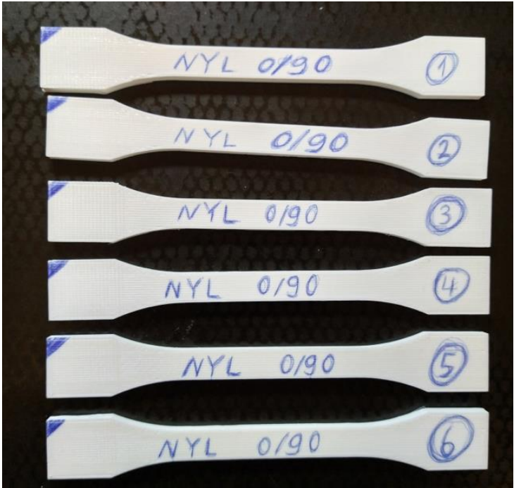
Figure E - 2: Printed "0°/90°" nylon specimens:
