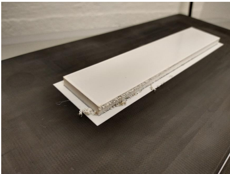
Figure 8-5: Fibre stringing observed on the complete printed sandwich panel specimens
