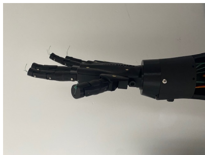
(c) Maximum pronation position of the prosthesis.
