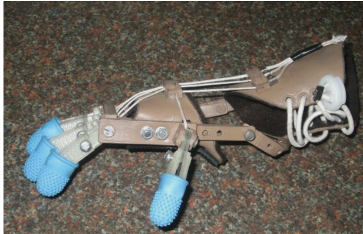
Figure 2.10: Design of the Robohand (adopted from [54]).
