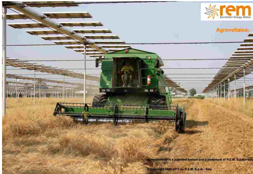
Figure 7: Overhead dynamic system in Italy © REM Tec
