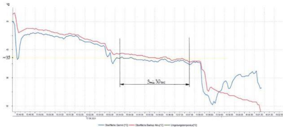
Figure 2.14 Garmin G5 in the oven with a relative humidity of about 80%
