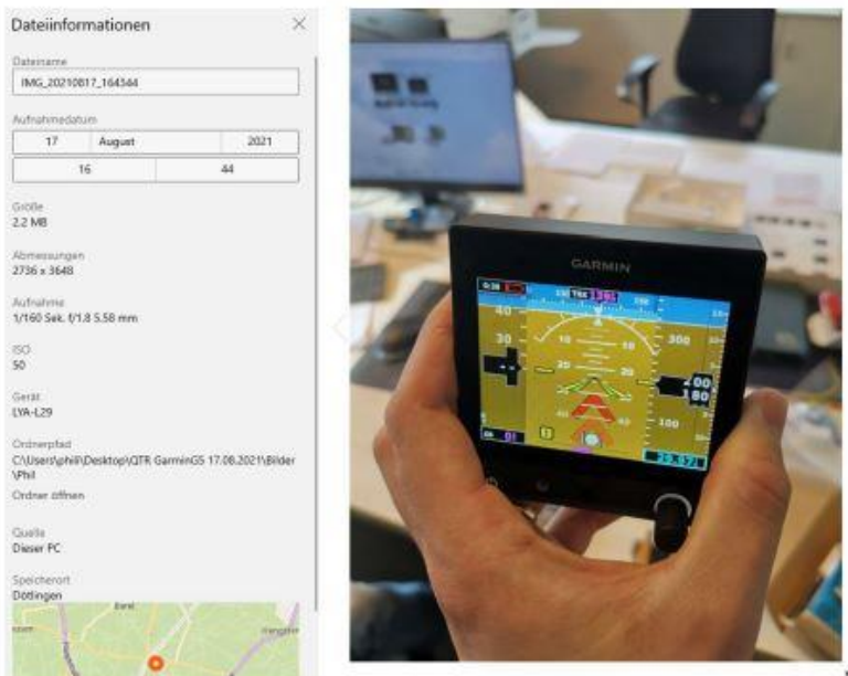
Figure 2.2 Garmin G5 at 16:44 with a with a remaining runtime of 38 min.
