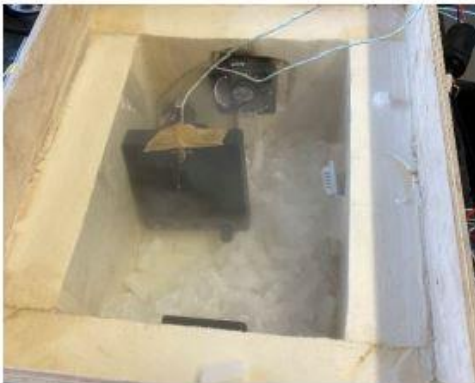
Figure 2.6 Garmin G5 in the insulated box with dry ice cooling
