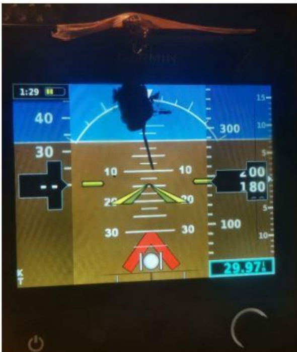
Figure 2.11 Garmin G5 in the oven at about 50 °C when switched on
