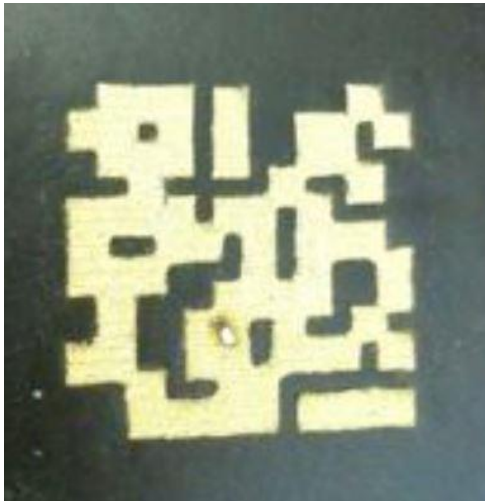
Figure 6.2 Genetically evolved patch antenna (Hope 2011, page 285)
