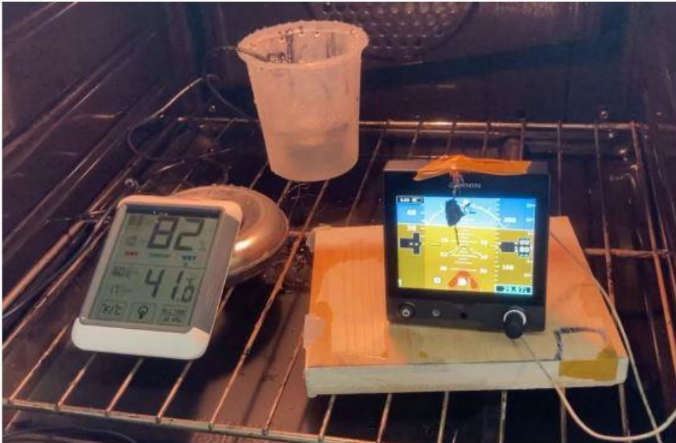
Figure 2.15 Video snapshot when opening the oven at 82% relative humidity at about 39 °C
