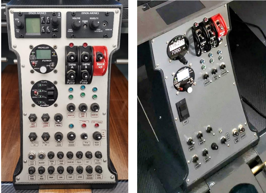
Figure 5.10 Flywhale panel with fuses (left) and Flywhale panel with VPX box installed (right)
