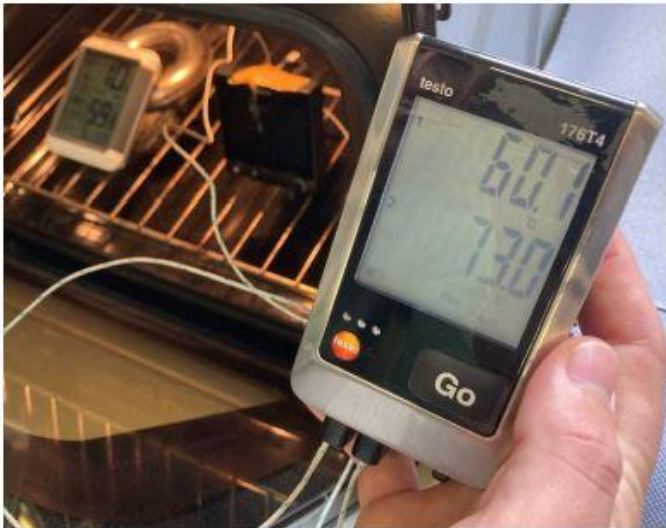
Figure 2.10 Garmin G5 in the oven at more than 60 °C
