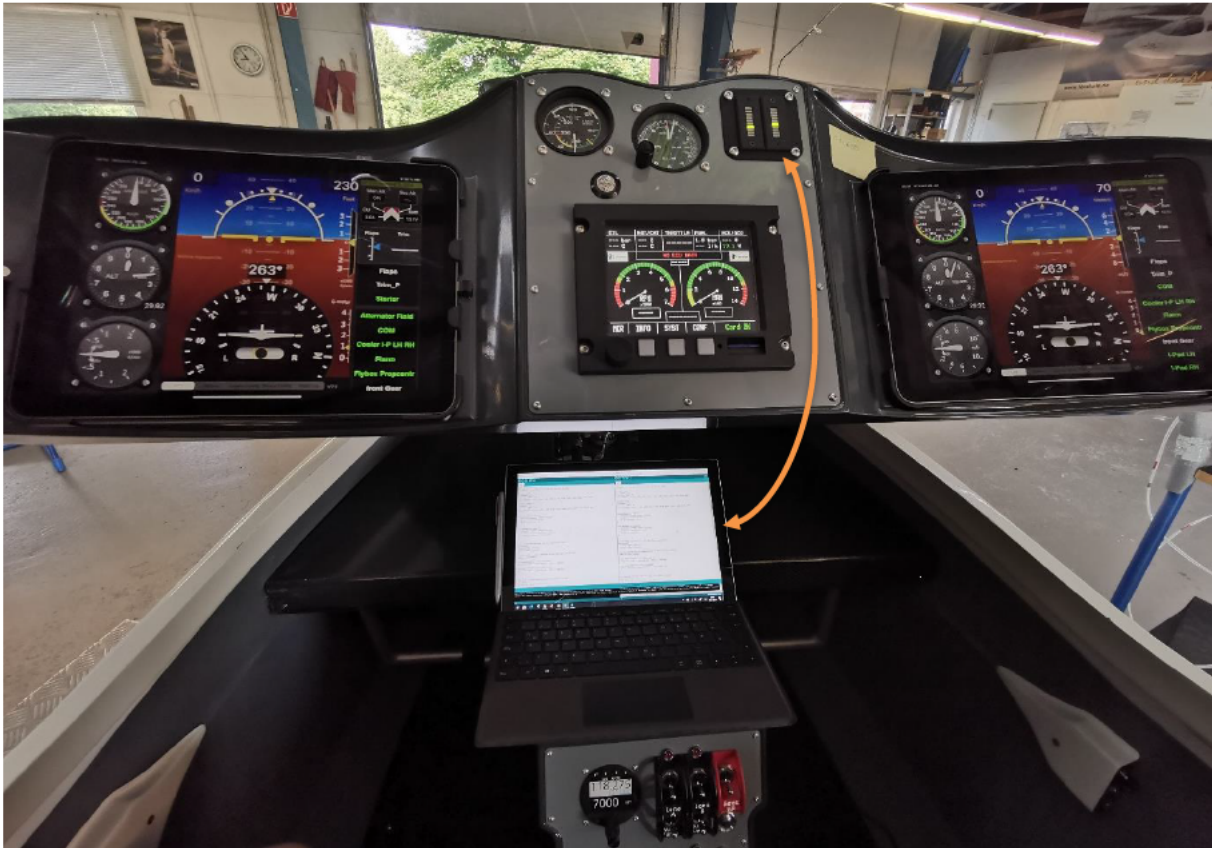
Figure 5.25 Cockpit of Flywhale Aircraft – last calibration of fuel level indicator in arduino code
