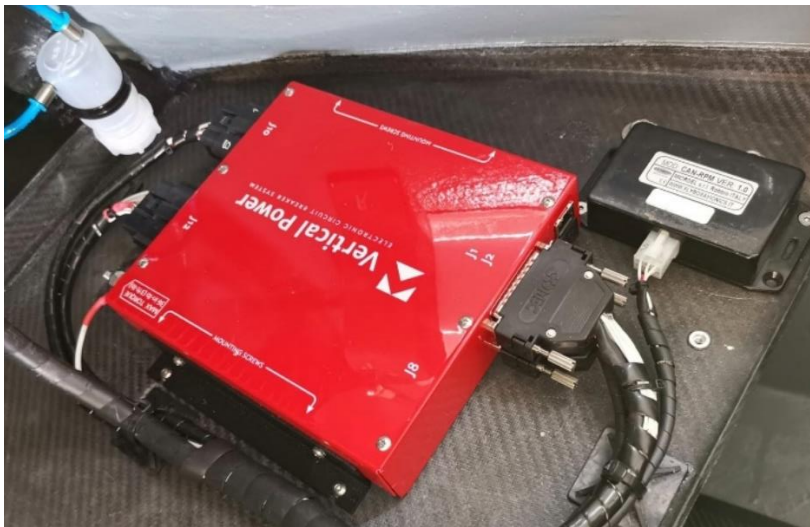
Figure 5.4 VP-X installed in the Flywhale
