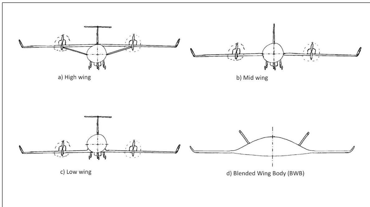
Figure 5.1 Wing configurations
