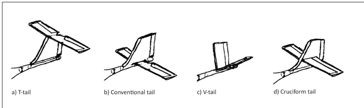
**Figure 5.2** Empennage configurations
