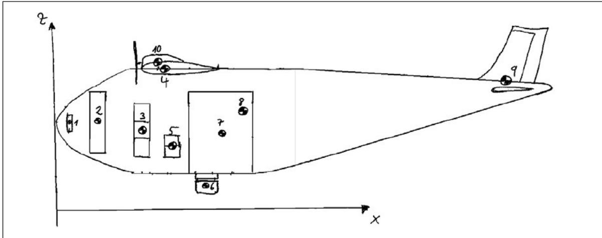
Figure 8.1 Assumed mass distribution of the design approach – side view
