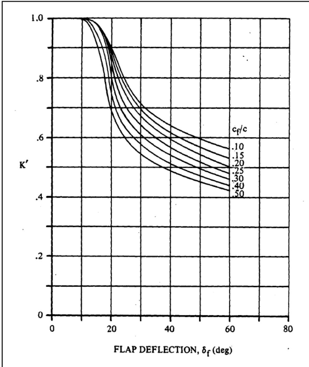
**Figure A.2** Empirical correction for nonlinear effect at bigger flap angles (Scholz 2015, Sec. 11.4, Fig. 11.17)
