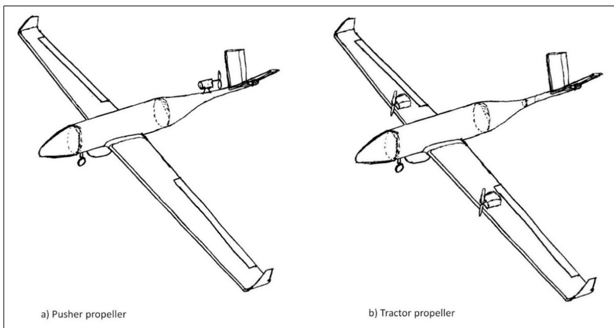
**Figure 5.3** Pusher and tractor propeller configurations
