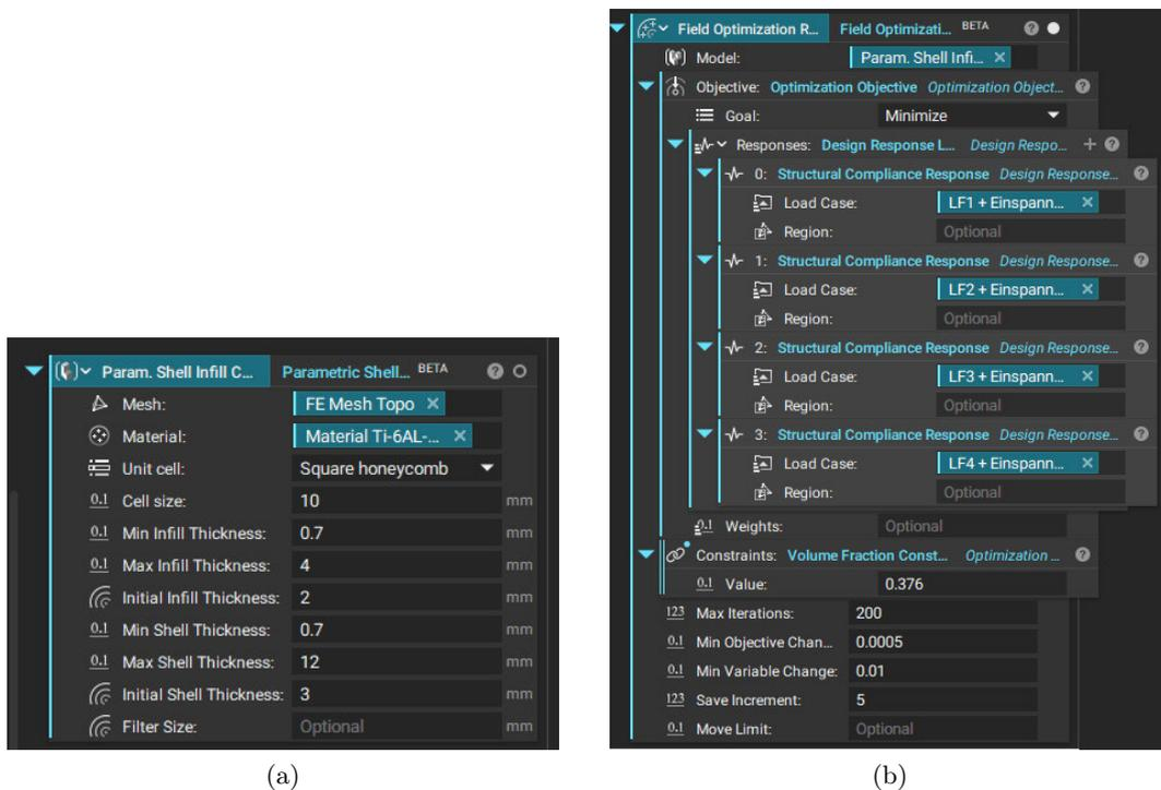
Abbildung 31: 31a Parametric Shell-Infill Block | 31b Fieldoptimization Block
