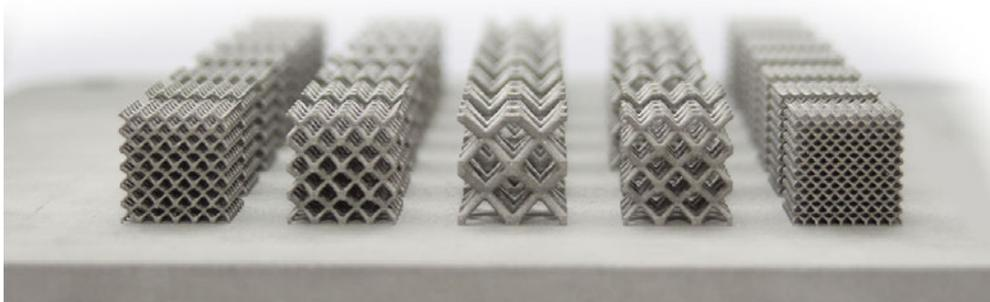
Abbildung 3: Lattice Teststrukturen at the University of Nottingham [4]
