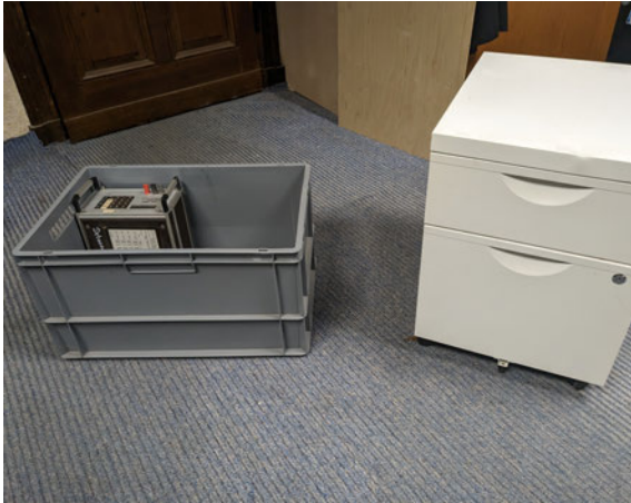
(a) Evaluated measurement setup consisting of a metal cabinet, a plastic storage box with a calibration source in a metal casing.
