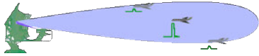
Figure 2.4: A rotating air surveillance radar using the directivity and therefore the radiated power in different directions to make conclusions about the azimuth of the target.
