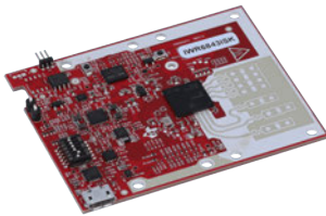
Figure 5.5: The IWR6843ISK module featuring three transmit and four receive antennas connected to a IWR6843 radar sensor.
