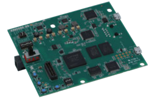
Figure 5.2: The DCA1000 evaluation module featuring a Lattice FPGA and GBit network interface for capturing ADC data directly over LVDS.
