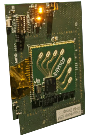
Figure 5.6: The custom radar module with the IWR6843 radar sensor. The orthogonal antenna rows are visible. The module is mounted on an adapter board for the DCA1000 evaluation module. It also features three TX antennas in the vertical direction and four RX antennas in the horizontal direction
