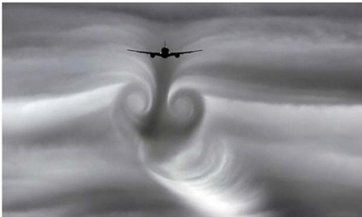
Figure 1: The vortex wake behind lifting wings descending through a thin cloud layer (Source: Airlines.net)
