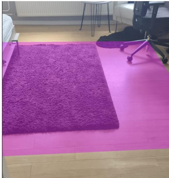
Figure 4.14: Rendered RANSAC plane with size of  $2 \cdot 2\text{m}$
