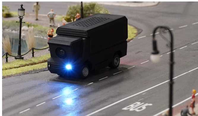
Figure 4.1: The tincar during a data collection test drive, remote controlled by a human, in the section of Knuffingen in the Miniatur Wunderland Hamburg. The car is equipped with a camera, LEDs for headlights, blinkers and taillights and is controlled by an ESP32 microcontroller. The cars body features a cyberpunk-inspired design, with only one headlight to break the symmetry.
