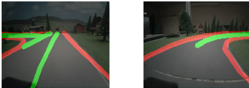
Figure 4.6: Two example images from the simulation’s camera feed are overlaid onto the corresponding frames captured by the real camera of the tinycar. Given that the simulated map mirrors the real environment in a 1:1 scale, the car is positioned at two random locations, and its orientation and position is determined using the tracking system. Subsequently, the camera images are simulated for these positions. The simulated images are then overlaid with the actual camera feed to verify the accuracy of the simulation parameters. Small differences in the positioning of the lane lines can be seen.
