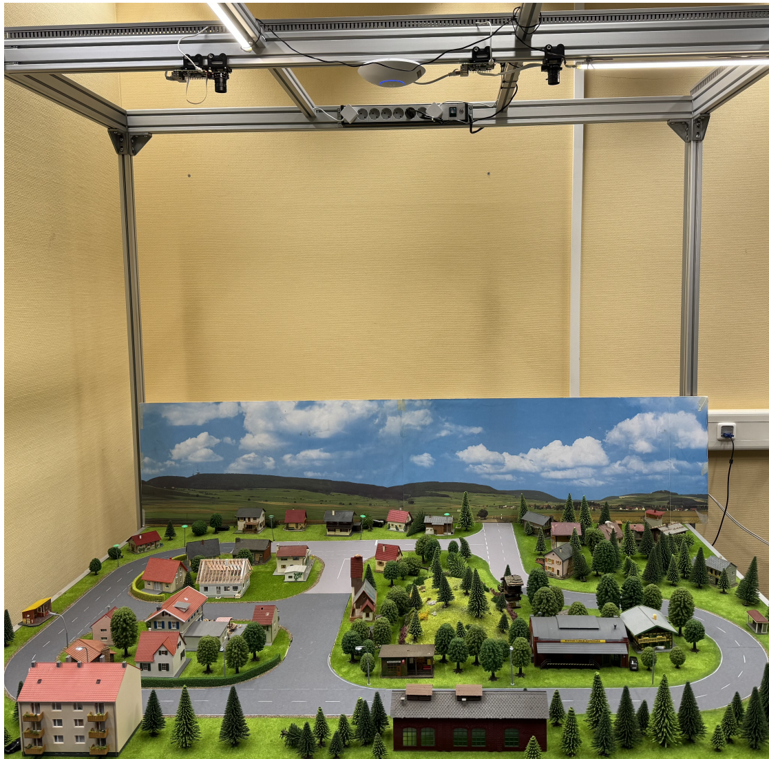
Figure 4.8: Overview of the environment at HAW Hamburg with the two tracking cameras mounted over the track. Each camera captures one half of the track. The cameras are directly connected to a Raspberry Pi 4 via the Camera Serial Interface (CSI), which processes the camera image and calculates the position and orientation of the car. The Raspberry Pi 4 is connected to the host computer via Ethernet. Between the two cameras sits the WiFi access point used to communicate with the car underneath.
