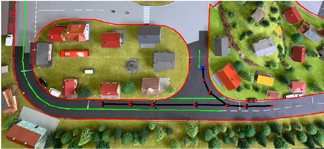
Figure 4.4: Example image of the mapbuilder tool. The tool is used to annotate the map of the environment. The mapbuilder generates a json file with graphs for each lane line and the ground truth trajectory. The lines are polylines, meaning nodes are connected by straight lines with no curvature. The reference image is only used for the tool and not part of the later generated map. The tool allows that paths can be split, needed for intersections on the ground truth trajectory.
