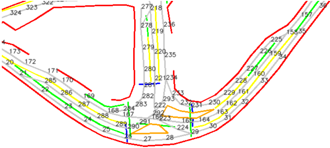
Figure 5.6: Part of the map of the Knuffingen environment with a large intersection. From each direction the intersection has a distinct lane for turning or keeping straight. This lane splitting happens centimeters before the actual intersection. It can be seen at node number 277, 21 and 158.
