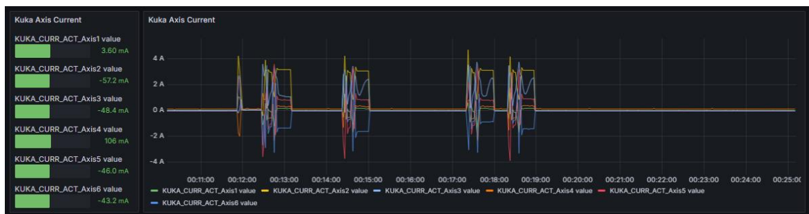
Figure 5.36: The current of each KUKA axis as an excerpt of its dashboard [67]
