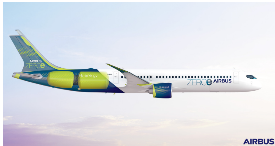
Figure 2.10: Airbus ZeroE conceptual aircraft with Hydrogen Tank(7)
