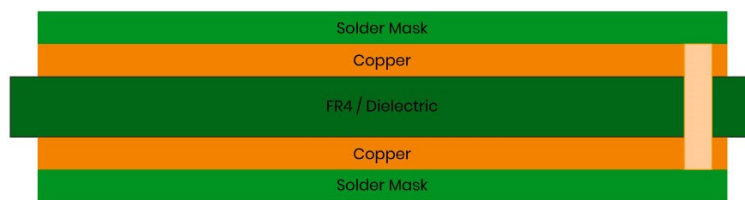
Figure 5.2: Two-layer PCB example extracted from [27]
