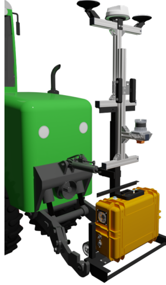
Figure 3.1: A graphical representation of the tractor with the sensor-box.
