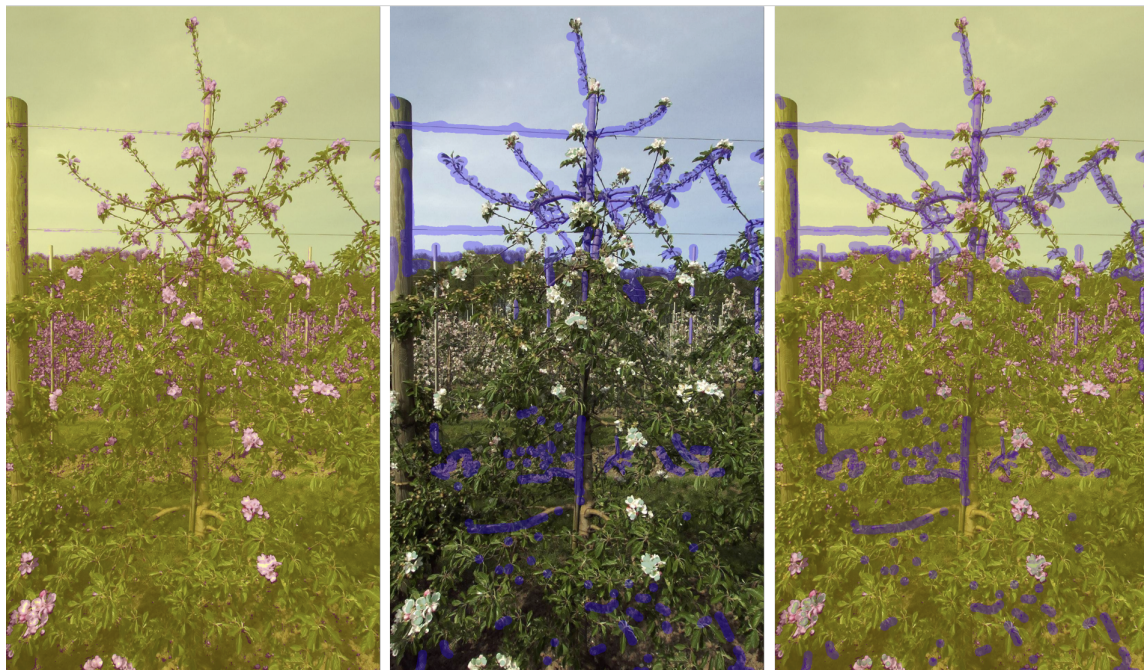
Figure 3.3: Example image from the assisted Labeling. Left: Image with machine predicted labels. Pink for Bloom and yellow for Not_Bloom . Middle: Image with human correction labels. Blue for Corrected_Not_Bloom and green for Corrected_Bloom . Right: Combination of both, which the model receives for further training.
