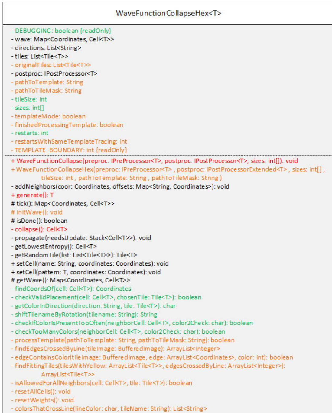
Figure 5.5: Class diagram for the WaveFunctionCollapseHex class. Methods and fields written in red are modified versions from the original WaveFunctionCollapse class. A green text color marks newly added parts. Black means unmodified. Orange are parts that are either modified or added but are only important for the template mode .
