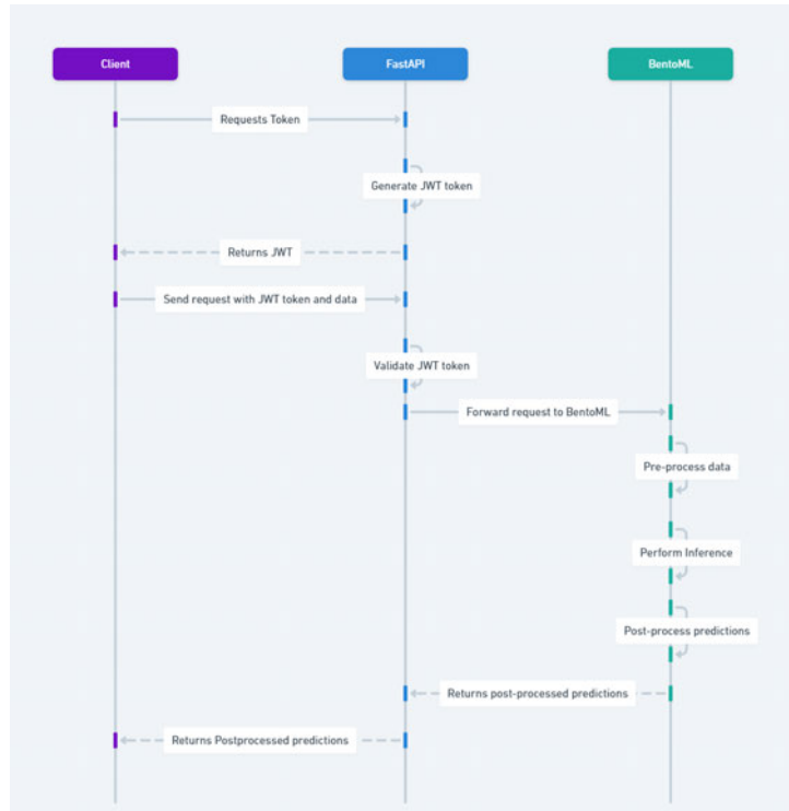
Figure 4.4: Client-Server Interaction Flow for BentoML with FastAPI setup
