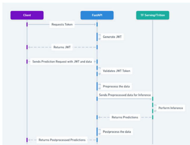
Figure 4.2: Client-Server Interaction Flow for TensorFlow Serving/Triton Inference Server Setup
