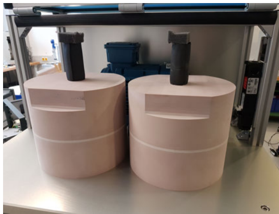
Figure 3.10: Cylindrical cover to insulate the bearing [31]
