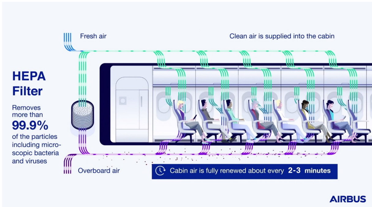
Figure 7: Airbus-Video "Cabin Air Flow". Shown is a longitudinal cut through the cabin along the aisle. Air is coming from above and below the overhead compartments. The air flows around the passengers (in contrast to Figure 5, where the air stays clear of the passengers) and leaves the cabin towards the cargo compartment ( https://youtu.be/rcfq9a1_27I ).
