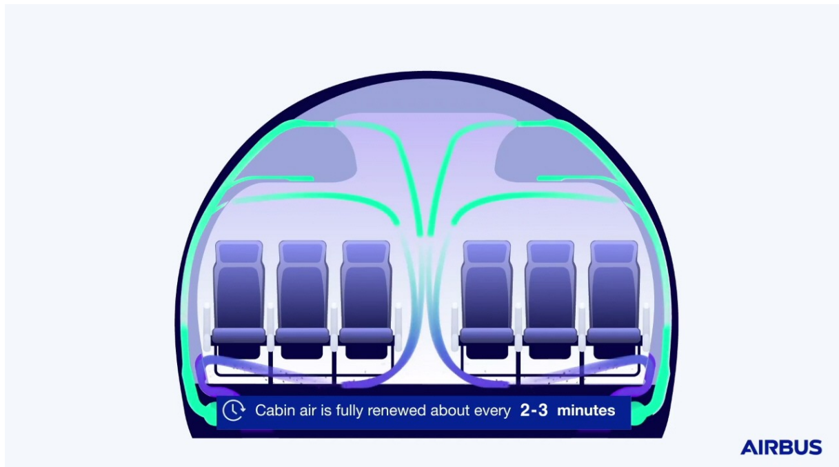
Figure 5: Airbus-Video "Cabin Air Flow". According to this figure, the air flow in the cabin cross section has its origins above and below the overhead compartments. The air descends in the aisle and leaves horizontally over the floor where it finds its way into the cargo compartment ( https://youtu.be/rcfq9a1_27l ).
